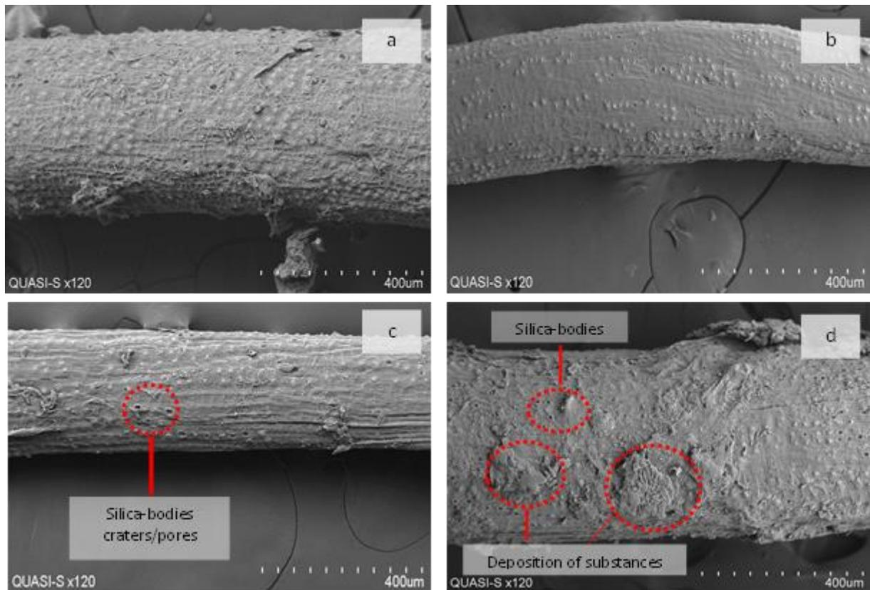
**Fig. 4.** SEM images of EFB fibre treated with (a) 0.2%, (b) 0.4%, (c) 0.6%, and (d) 0.8% NaOH at 120x magnification
