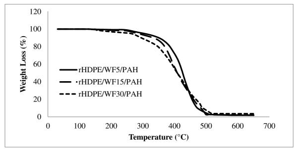
**Figure 4:**Thermogravimetric curves of rHDPE/WF/PAH composites at different fiber loading.
