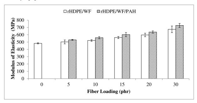
**Figure 2:**Modulus of elasticity versus filler loading of rHDPE/WF and rHDPE/WF/PAH composites.
