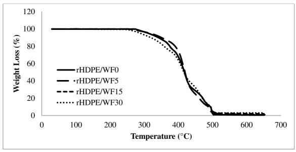
Figure 3:Thermogravimetric curves of rHDPE/WF composites at different fiber loading.
