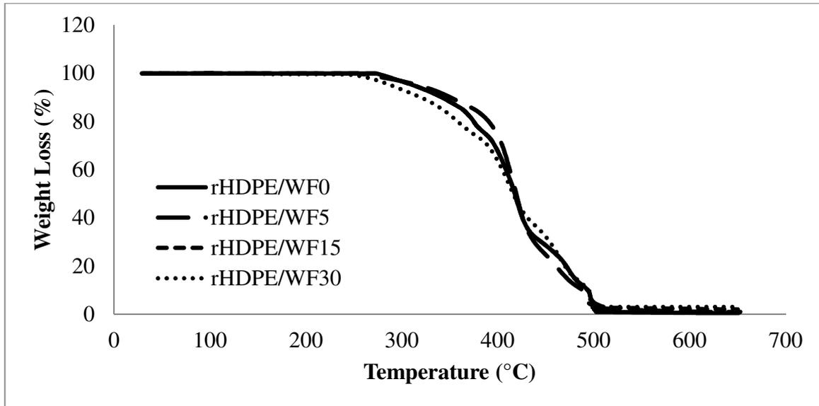
**Figure 3:** Thermogravimetric curves of rHDPE/WF composites at different fiber loading.
