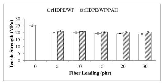
**Figure 1:**Tensile strength versus fiber loading of rHDPE/WF and rHDPE/WF/PAH composites.
