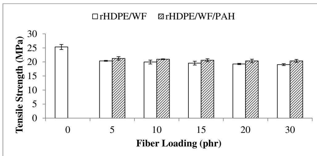
**Figure 1:** Tensile strength versus fiber loading of rHDPE/WF and rHDPE/WF/PAH composites.
