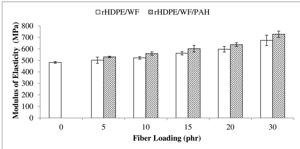
**Figure 2:** Modulus of elasticity versus filler loading of rHDPE/WF and rHDPE/WF/PAH composites.
