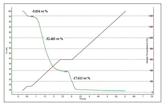
Figure 4:TGA results for sewage sludge
