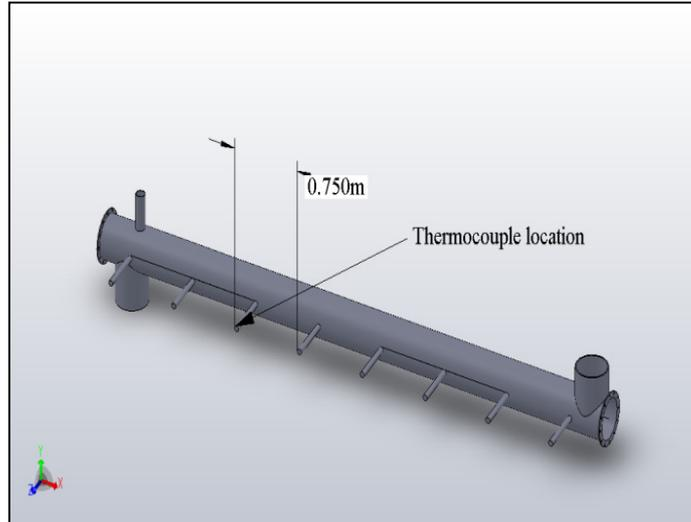
**Figure 2:** Thermocouple location along the dryer
