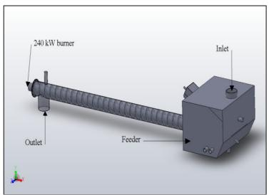
Figure 1:Schematic of the thermal dryer
