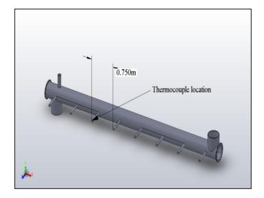
Figure 2: Thermocouple location along the dryer
