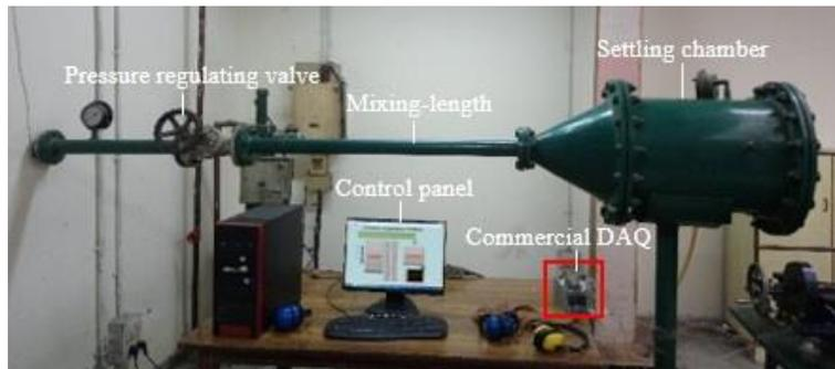
**Fig. 1.** 75 mm diameter pipe connected from storage tanks, followed by a pressure regulating valve, mixing length, wide-angle diffuser and settling chamber
