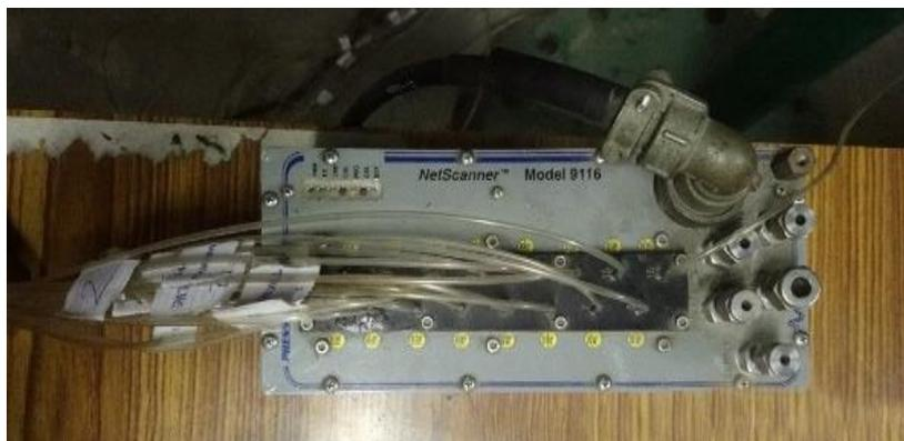
**Fig. 2.** Pressure Systems NetScanner™ Model 9116 Pressure Transducer
