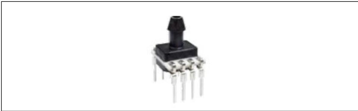
**Fig. 6.** HSC Series TruStability® Pressure Sensor, DIP package, AN single-axial, barbed-port, analog output type, 10% to 90% of  $V_{supply}$  transfer function, 5V DC supply voltage [12]
