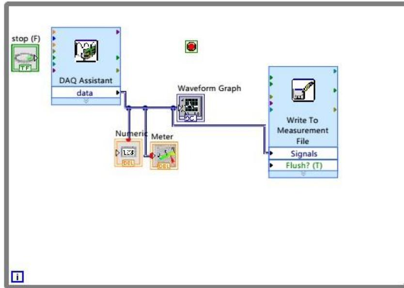
Fig. 11. LabVIEW™ DAQ – Process flowchart
