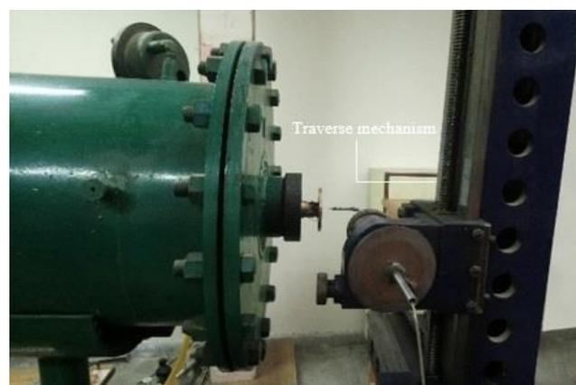
**Fig. 4.** Nozzle calibration setup
