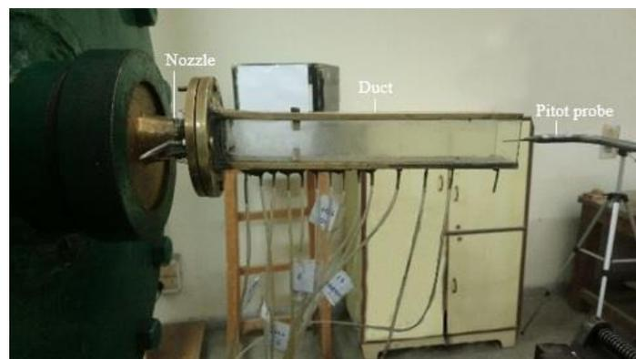
**Fig. 3.** Nozzle connected to the duct by flanges with a pitot probe at the duct exit, fixed to the traverse mechanism
