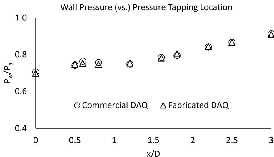
Fig. 14. Wall pressure data validation for  $L/D = 6$
