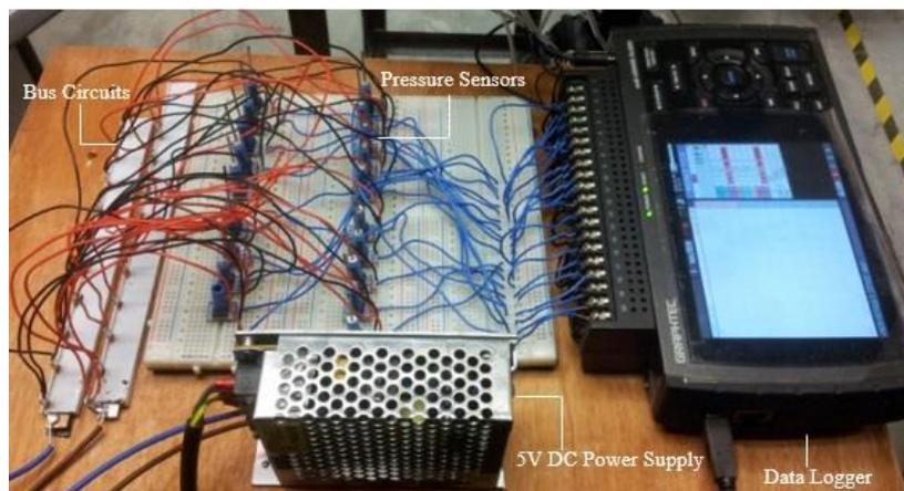
Fig. 9. Cost-effective DAQ instrumentation
