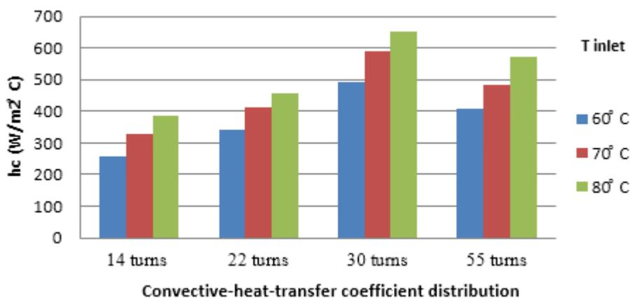
**Fig. 4.** The coefficient distribution of convective heat transfer  $h_c$  to the length of the HE tube pass
