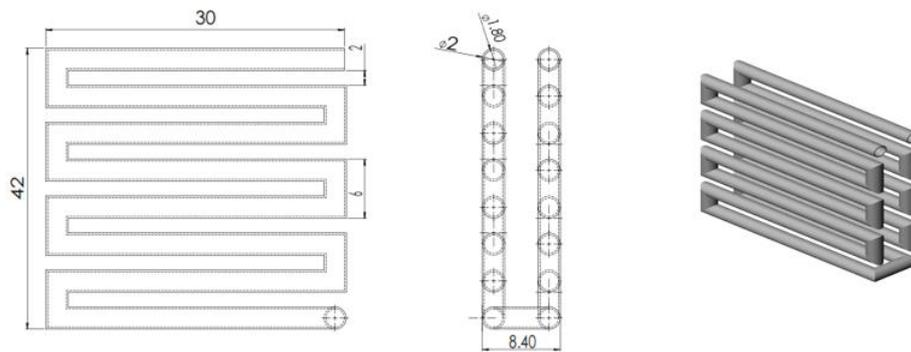
**Fig. 1.** Heat Exchanger Scheme tested
