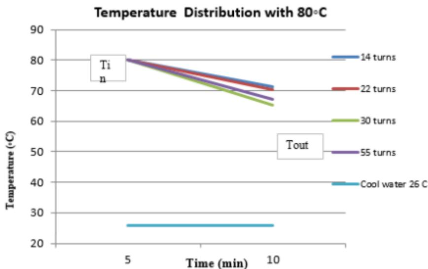
Fig. 2. Temperature distribution of tube cooling with 80°C inlet temperature for U-HE Turning Variations
