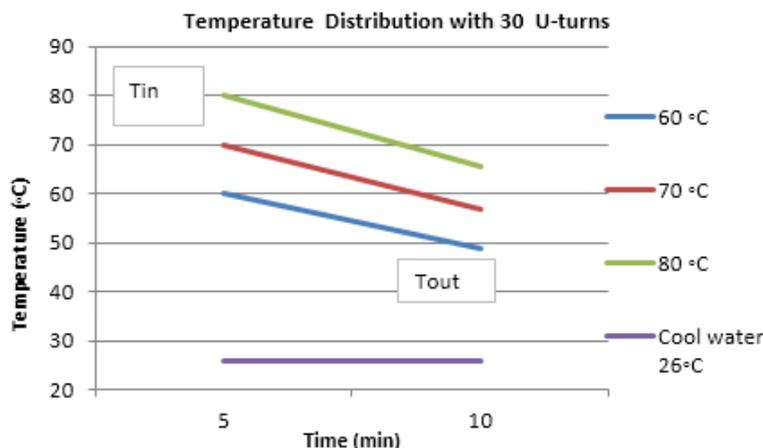
**Fig. 3.** HE Temperature Distribution of 30 Cm long pass and 30 turns with temperature entering tube 60°C, 70°C and 80°C
