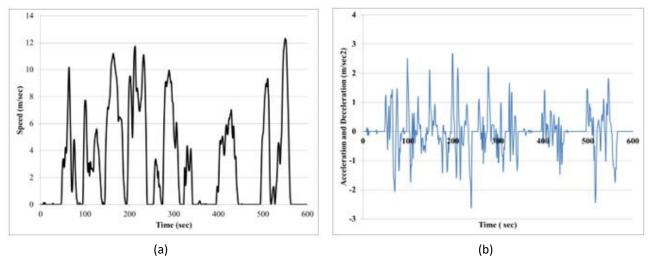
Fig. 4. (a) and (b) represent the standard driving cycle and acceleration/deceleration in New York city
