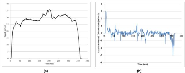
Fig. 3. (a) and (b) represent the standard driving cycle and acceleration/deceleration on Highway
