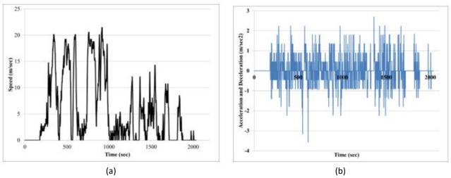
Fig. 5. (a) and (b) represent the real world driving cycle and acceleration/deceleration cycle in Baghdad
