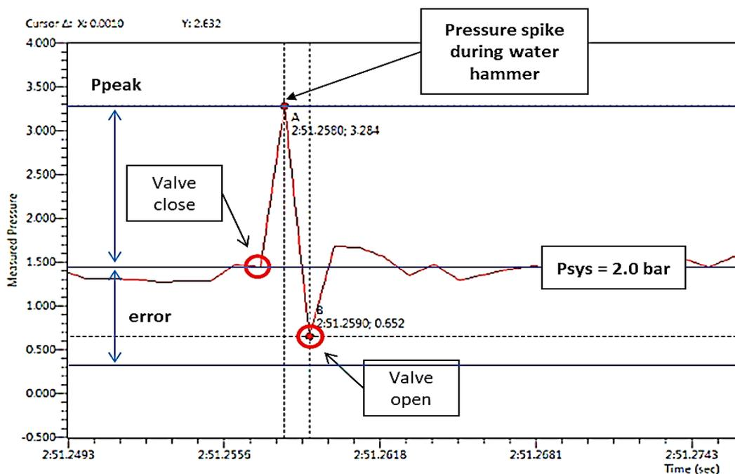
Fig. 5. Graph for Actual Pressure of Water Hammer
