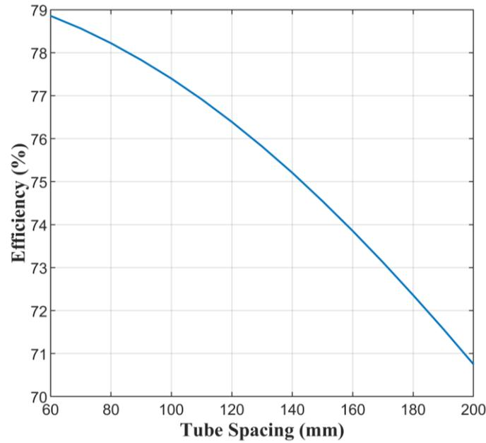
**Fig. 6.** Variation of energy efficiency versus tube spacing
