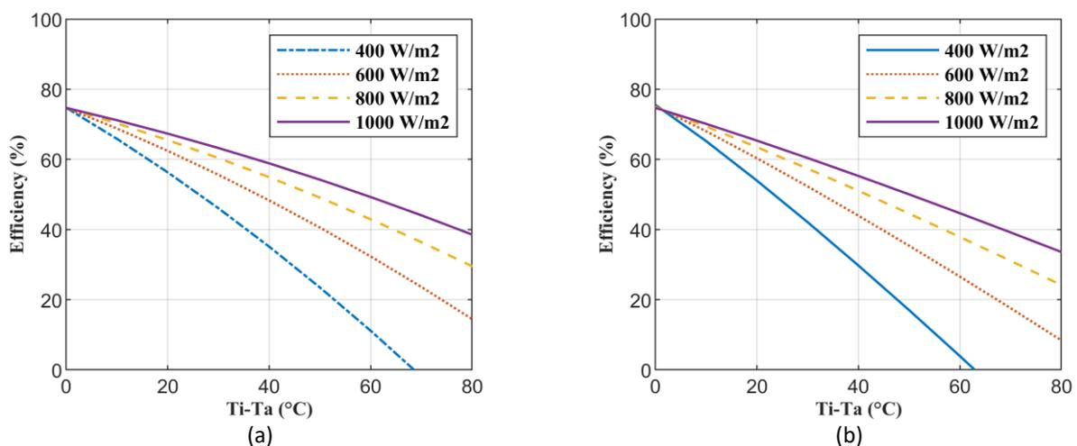
**Fig. 1.** Efficiency curve with temperature difference under various solar radiation intensity (a) Experimental results of [41]; (b) Simulation Result of this work
