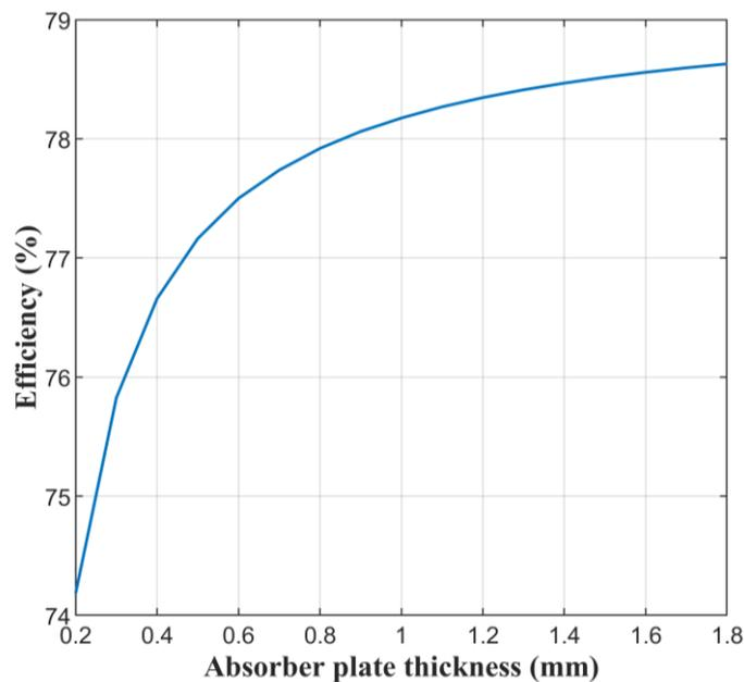
**Fig. 4.** Variation of energy efficiency versus absorber plate thickness
