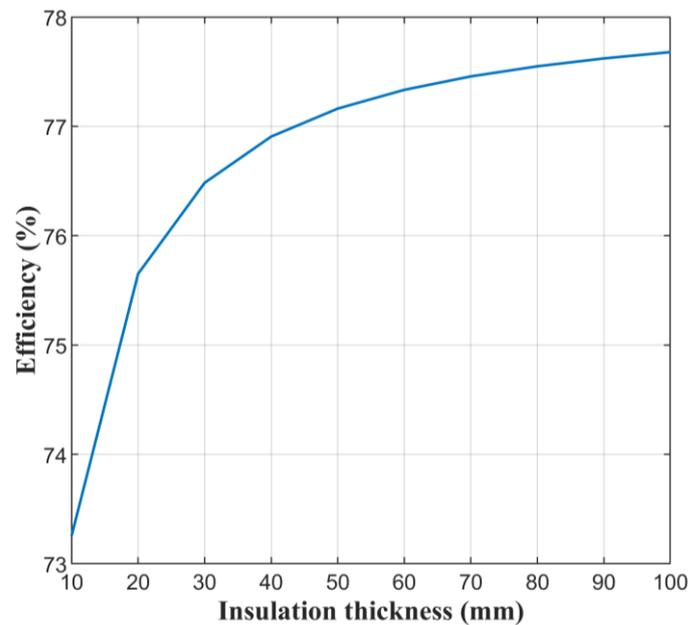
**Fig. 7.** Variation of energy efficiency versus insulation thickness
