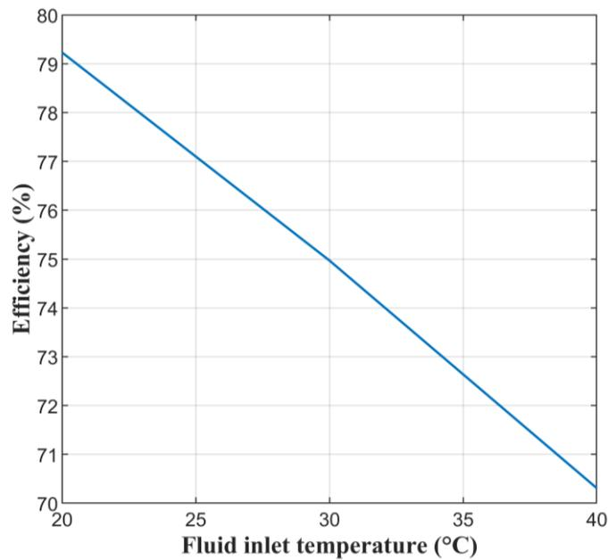
**Fig. 3.** Variation of energy efficiency versus fluid inlet temperature
