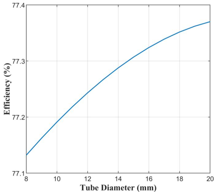
Fig. 5. Variation of energy efficiency versus tube diameter
