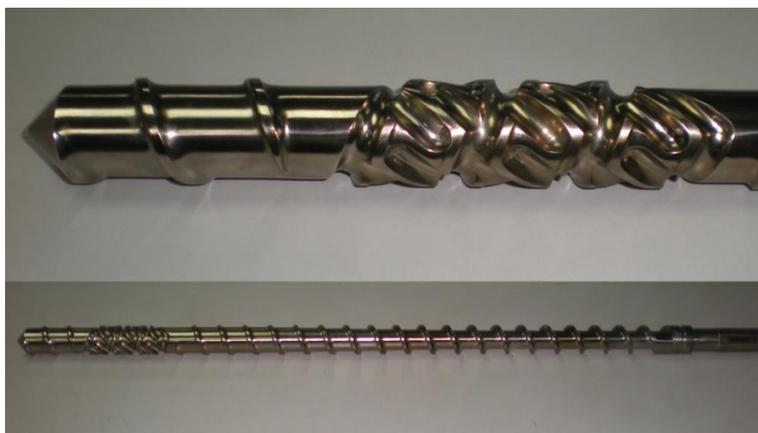
**Fig. 1.** Single screw extruder with special design nano-mixer
