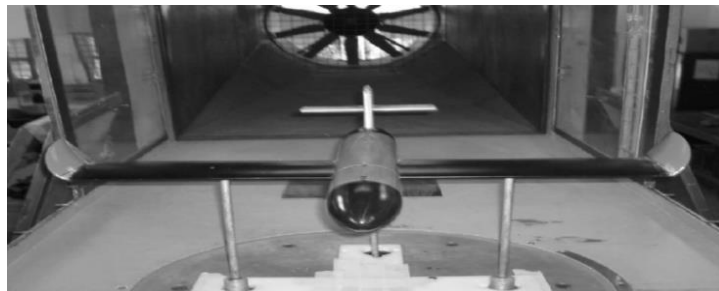
Fig. 8. Wind tunnel setup of blended elliptical winglet [50]
