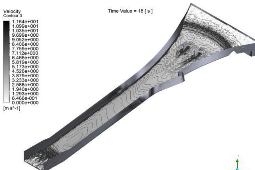
Fig. 7. Velocity contour along the spillway
