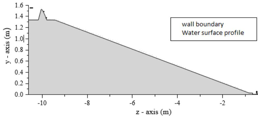
Fig. 6. Water surface profile along the spillway
