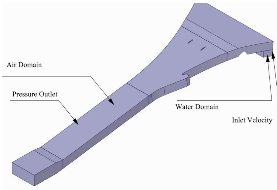
**Fig. 4.** Volume domain and boundary condition
