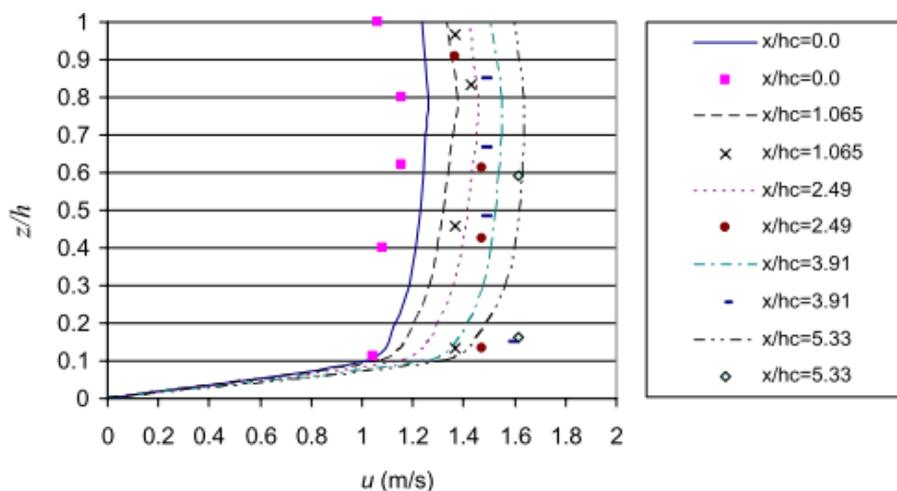
Fig. 12. Velocity profiles at multiple locations along the chute spillway [8]
