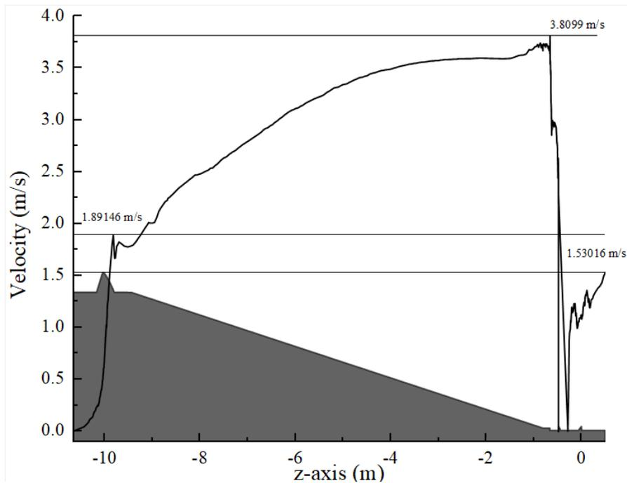
**Fig. 8.** Surface velocity profiles along the spillway
