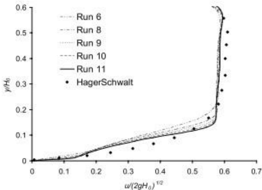
Fig. 11. Velocity profiles on the flat rectangular flume after the weir [19]
