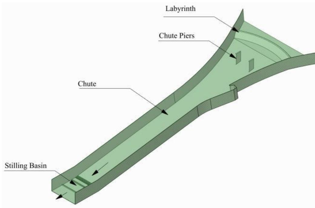
Fig. 1. Detail of spillways geometry
