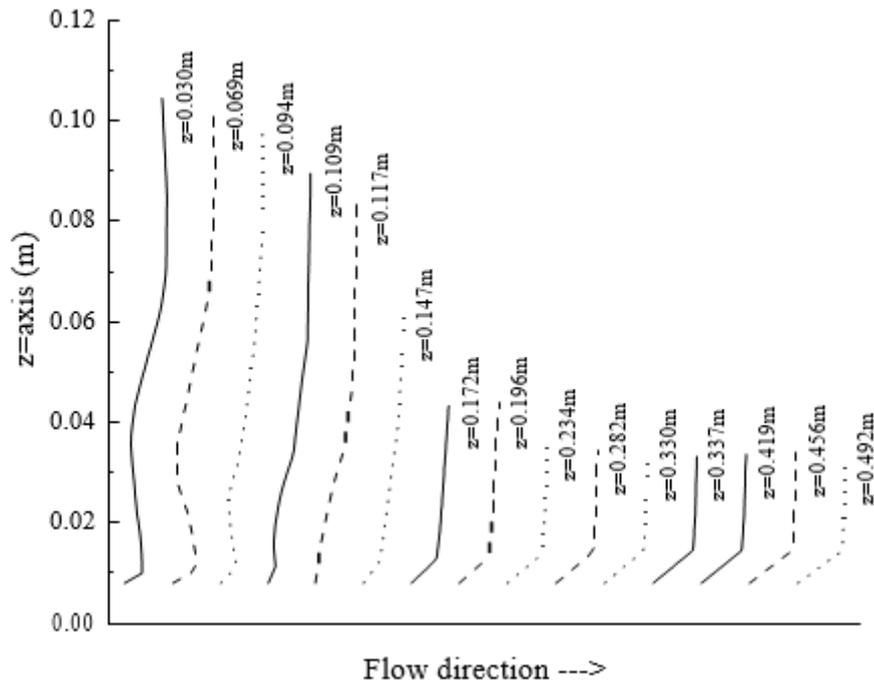
Fig. 10. Velocity profiles from  $z = 0.030 \sim 0.492\text{m}$
