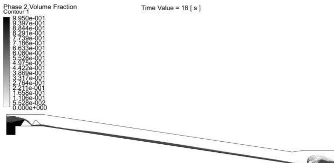
**Fig. 5.** Midplane volume fraction contour of the spillway
