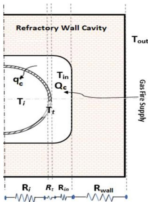
**Fig. 2.** Schematic representation of the Pyrolysis Furnace [22]
