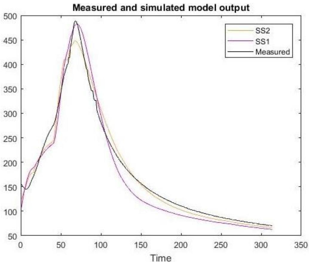
**Fig. 7.** Graph Showing the measured Output Y1 (T2) plotted with the Simulated Output using State Space Models 1 (SS1) and 2 (SS2) against Pyrolysis Time (t)
