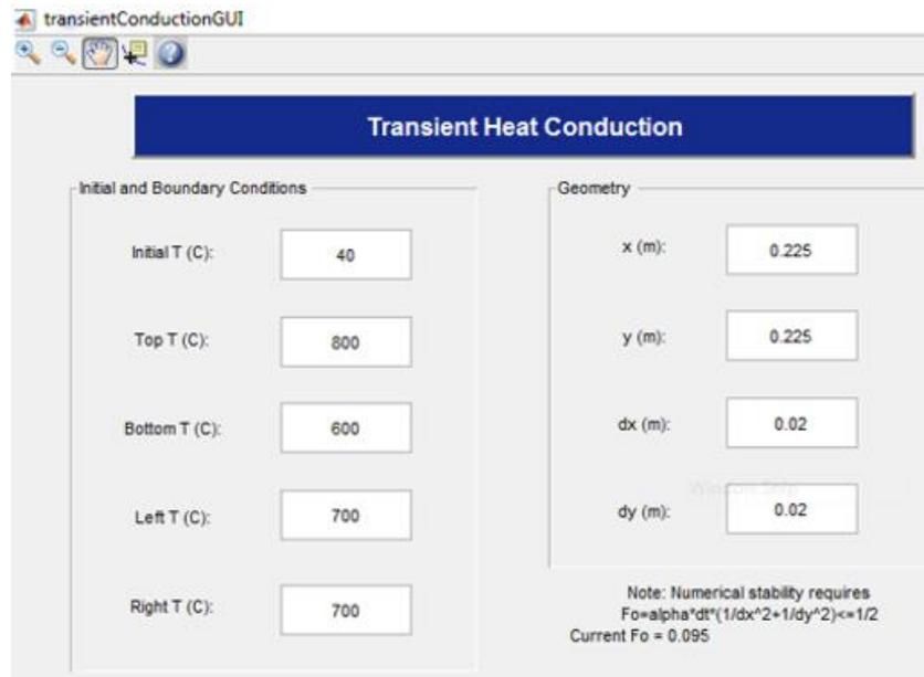
**Fig. 5.** GUI for setting boundary conditions transient heat conduction of the pyrolysis furnace
