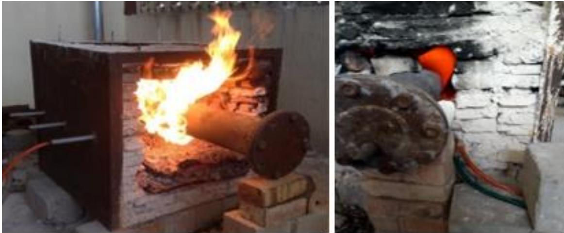
**Fig. 4.** Test-Running the model pyrolysis furnace [35]
