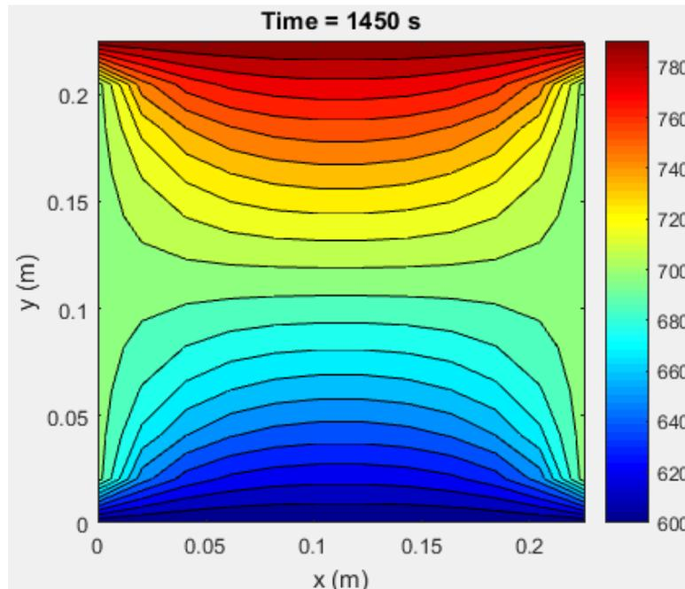
**Fig. 8.** Graph Showing the snapshot of heat transfer over x and y directions representing a specific temperature distribution pattern in the pyrolysis furnace at a pyrolysis time,  $t = 1450$  seconds
