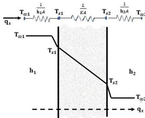
**Fig. 3.** 1D Heat transfer model prediction through the pilot furnace refractory wall; showing both the temperature profile and the equivalent thermal circuit [32]
