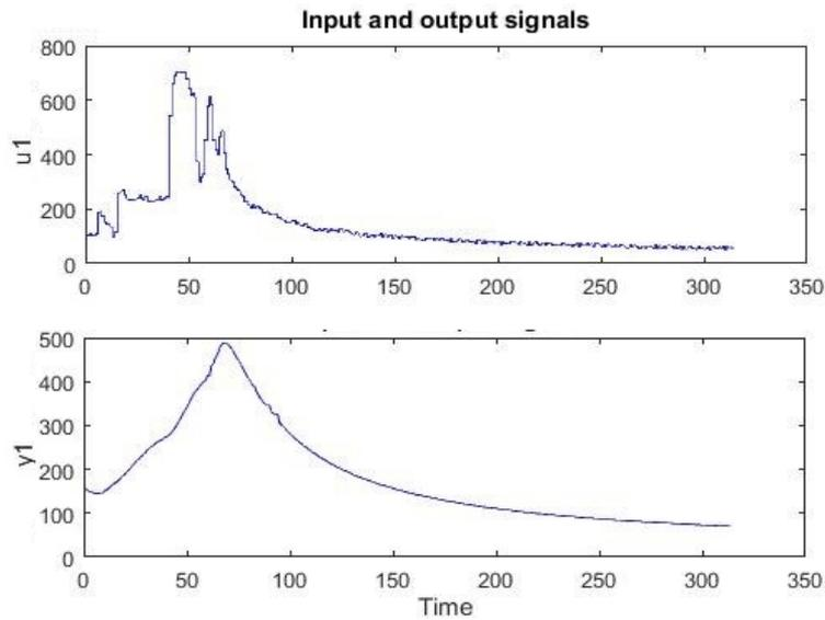
**Fig. 6.** Graph Showing a cumulative of Input U1 (T1) and Output Y1 (T2) Signal over four runs of fast Pyrolysis process against Pyrolysis Time (t)
