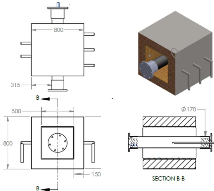
Fig. 1. Technical drawing of the model pyrolysis furnace [22]
