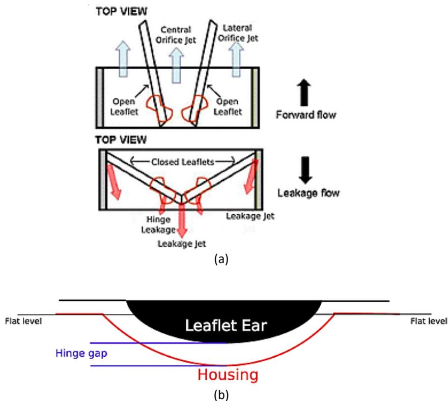
**Fig. 3.** Schematics of SJM valve (a) The SJM valve for forwarding flow and leakage flow and (b) Diagram of leaflet ear at the hinge recess housing [21]
