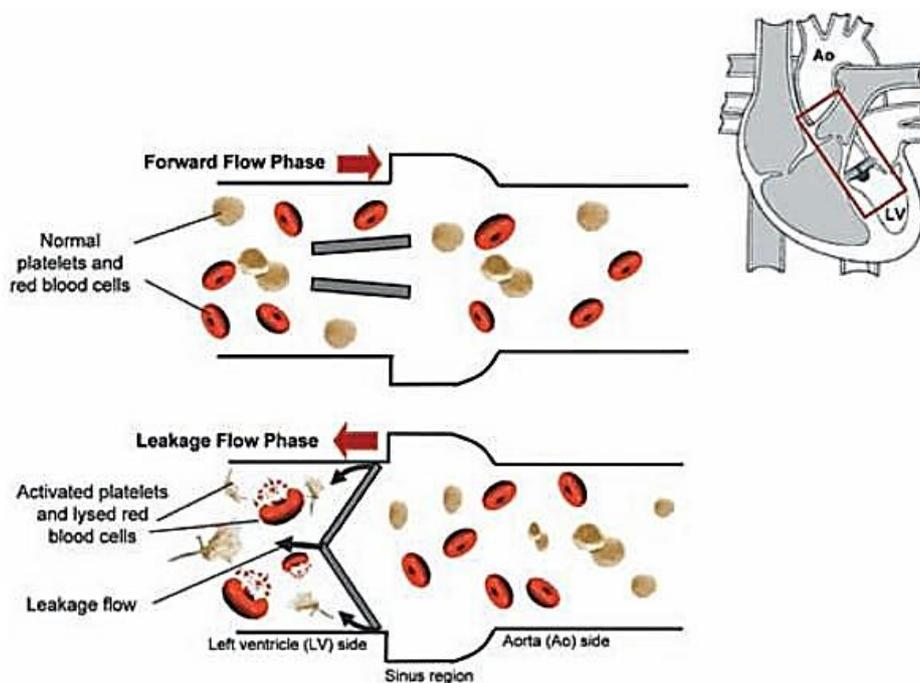
Fig. 7. The BMHV schematic throughout the leakage flow phase [44]
