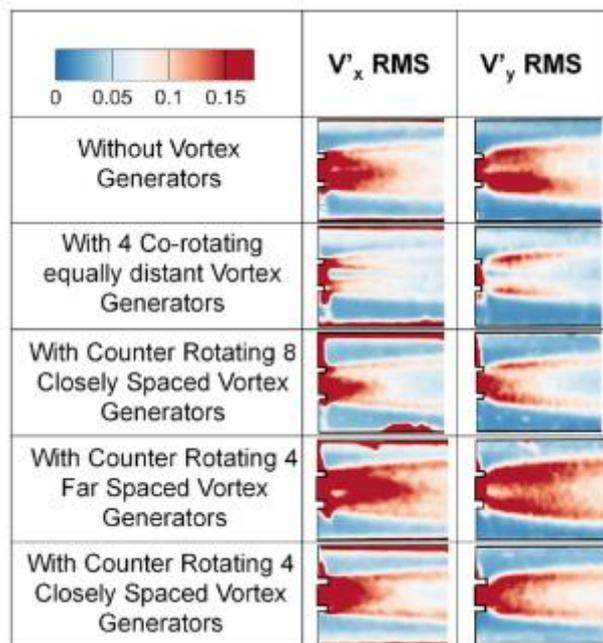
**Fig. 10.** RMS of the variation in velocity ( $V'_x$  and  $V'_y$ ) at peak systole for the particular valve cases [89]
