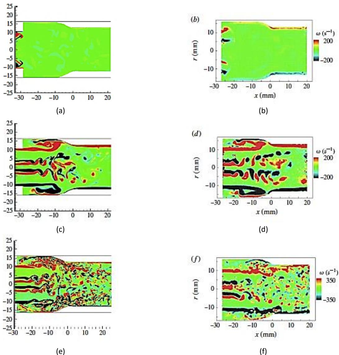
**Fig. 5.** The comparison of 2D vorticity magnitude between the simulation and experiment of BMHV flow: (a) opening, computational; (b) opening, experimental; (c) acceleration, computational; (d) acceleration, experimental; (e) peak, computational; (f) peak, experimental [28]
