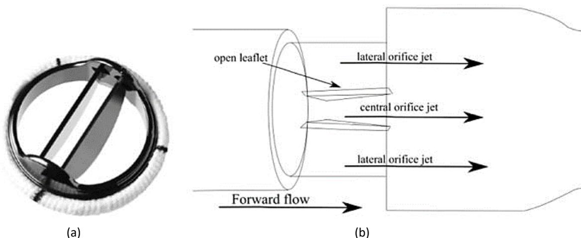
**Fig. 2.** SJM valve showing (a) Geometry of the SJM valve, (b) The forward flow characteristic [12]
