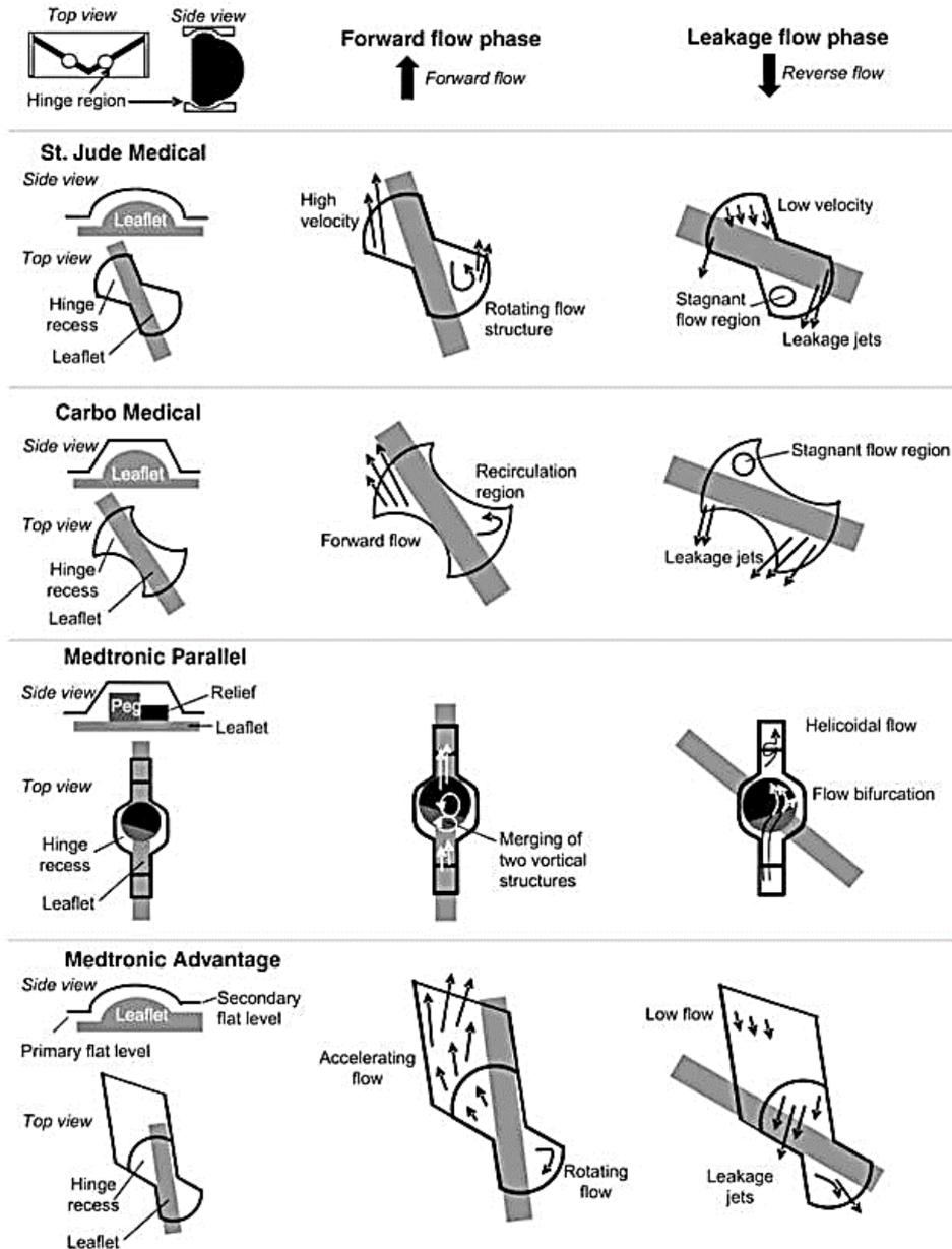
**Fig. 4.** The convolution flow fields in four hinge designs [11]
