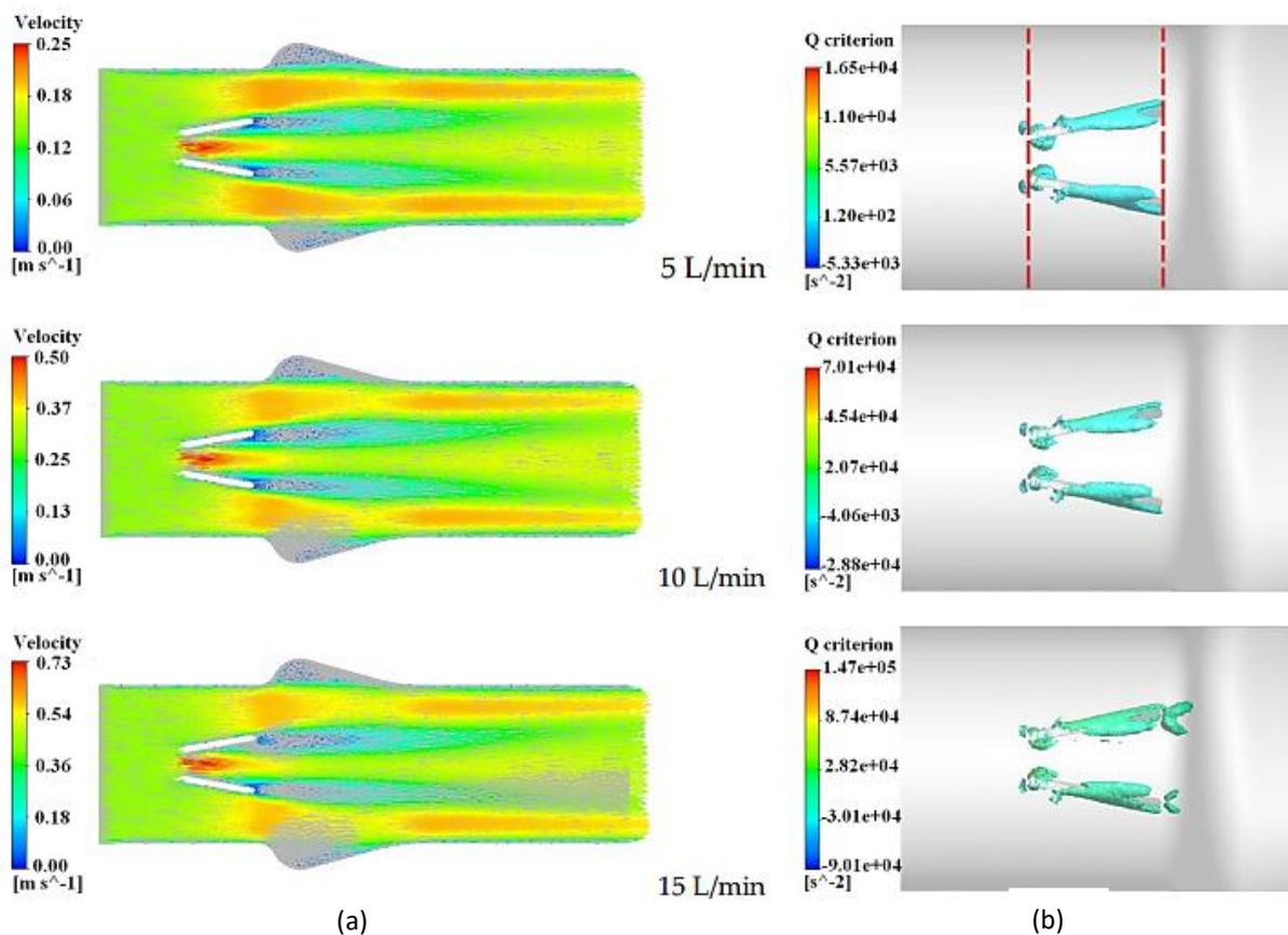
**Fig. 8.** Velocity distribution and Q criterion of the vortex core region of BMHV. (a) Velocity vector distribution and (b) Q criterion of the vortex core region [62]
