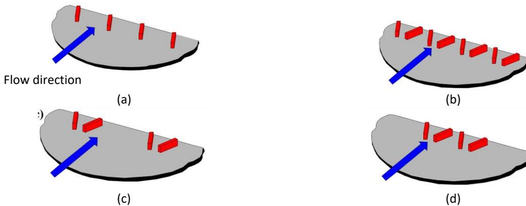
**Fig. 9.** The schematic of vortex generator arrangement: (a) co-rotating, (b) 8 equally spaced counter-rotating vortex generator, (c) 4 far spaced counter-rotating VGs and (d) 4 closely spaced counter-rotating VGs [89]
