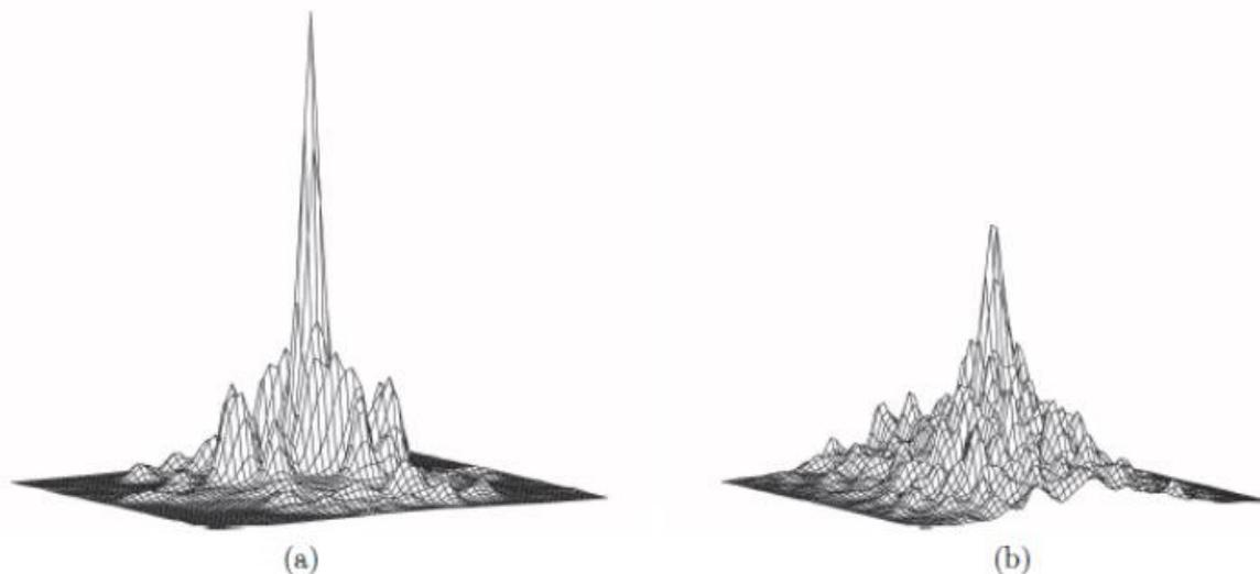
**Fig. 11.** A demonstration of the effects of displacement gradients on the correlation peak. The correlation of synthetic images with constant parameters show the difference between applying (a) no gradient and (b) a 0.2 pixels/pixel gradient [38]
