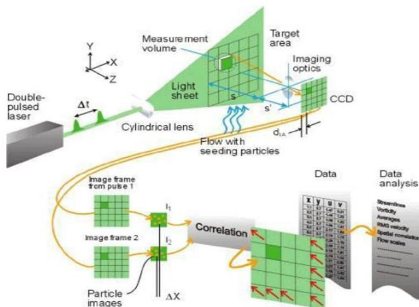
Fig. 2. Experimental arrangement for particle image velocimetry [6]
