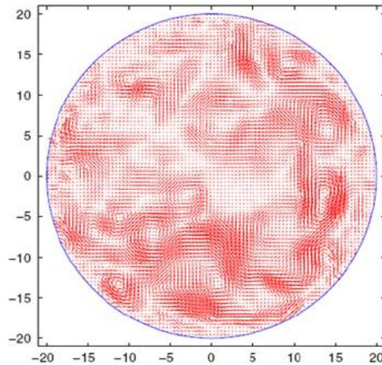
**Fig. 8.** Example of the instantaneous turbulent flow field in a cross-section of the pipe. Displayed resolution is  $8 \times 8$  px, or  $0.5 \times 0.5$  mm<sup>2</sup> [22]
