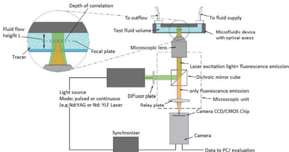
**Fig. 7.** Schematic of a  $\mu\text{PIV}$  [21]
