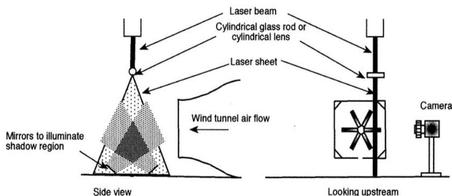
**Fig. 1.** Typical PIV experimental arrangement used in wind tunnel [4]
