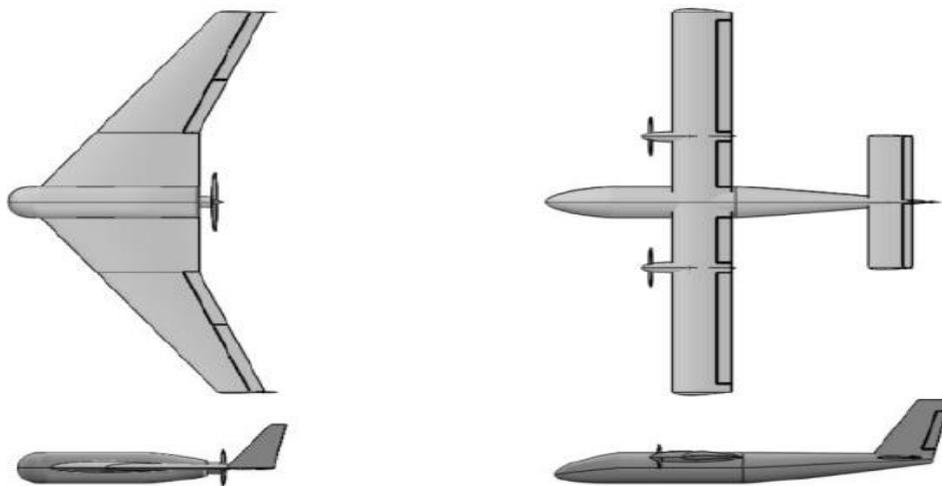
**Fig. 4.** BWB Baseline-IX (left) versus DHC-6 Twin Otter transport aircraft (right)
