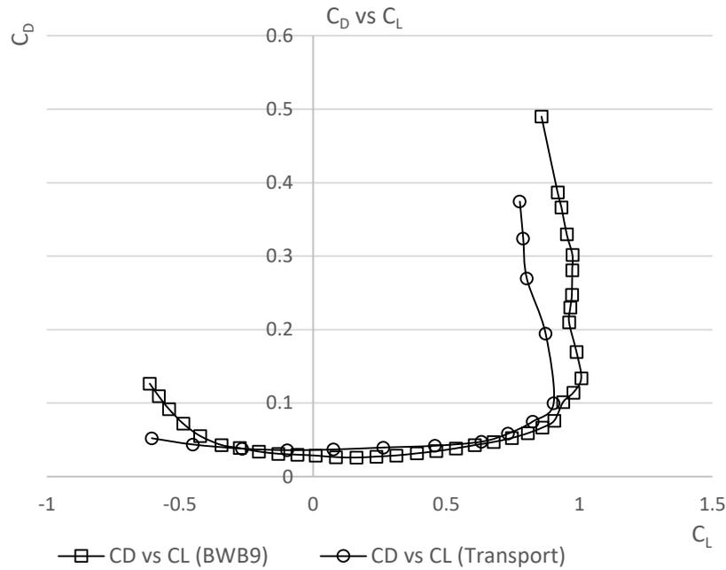
**Fig. 12.** Drag coefficient ( $C_D$ ) versus lift coefficient ( $C_L$ )
