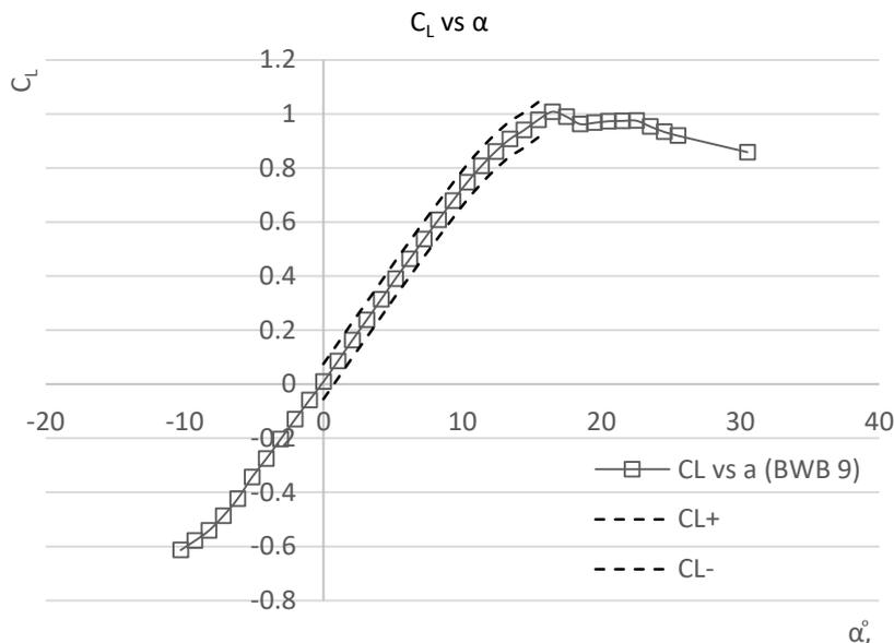
**Fig. 16.** Graph of lift coefficient versus angle of attack with accuracy tolerance region
