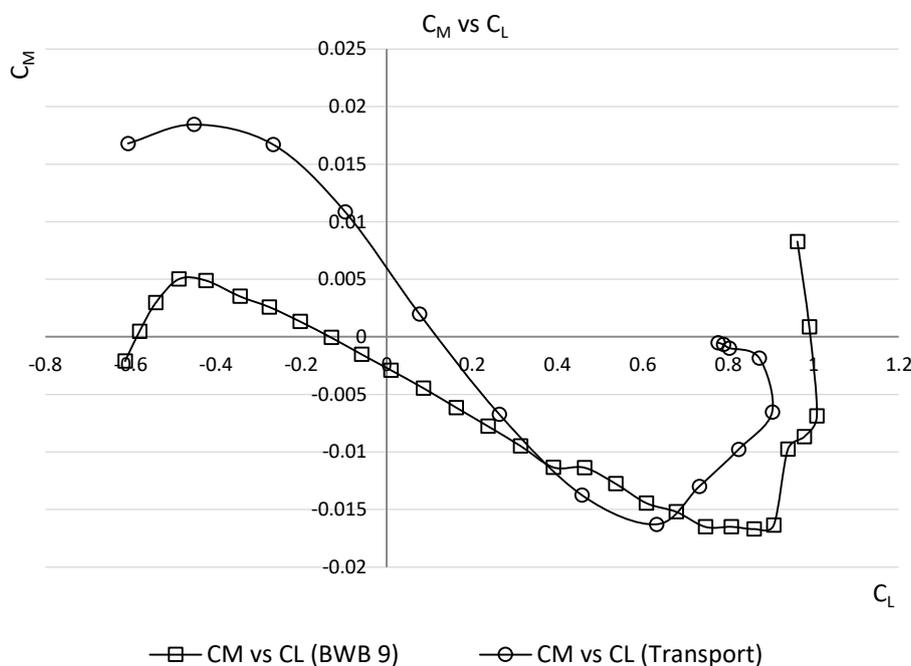
**Fig. 15.** Pitch moment coefficient ( $C_M$ ) versus lift coefficient ( $C_L$ )
