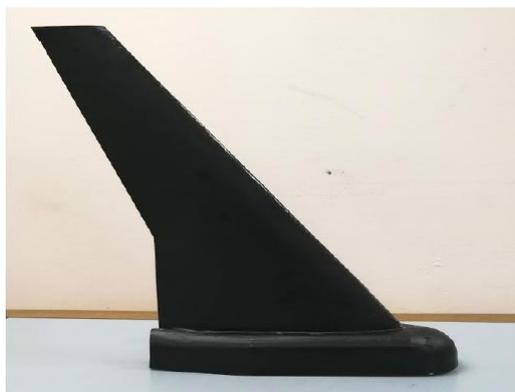
**Fig. 8.** BWB Baseline-IX wind tunnel model
