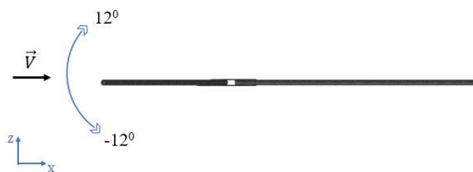
Fig. 3. Angles of tri-copter's frame are investigated
