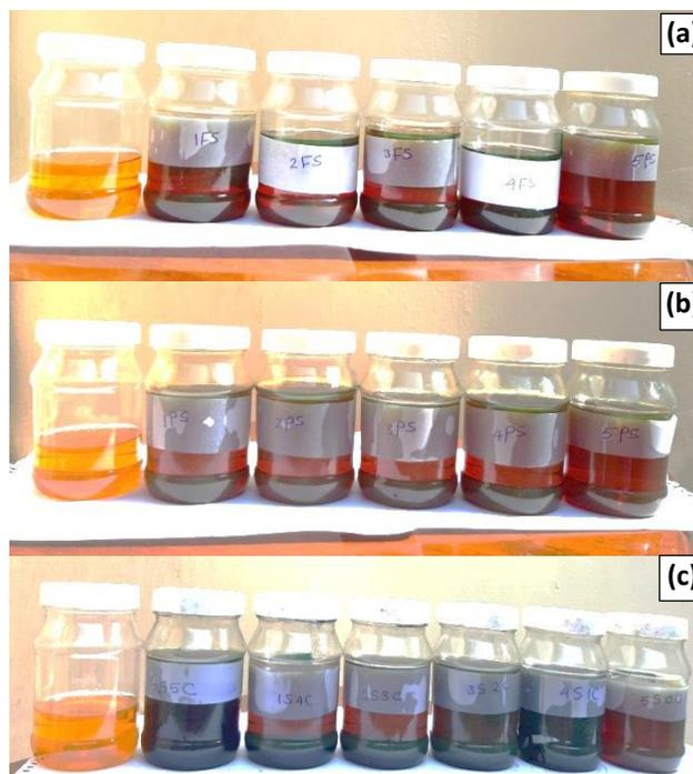
**Fig. 3.** The nanofluid samples; (a) Fumed silica nanofluid, (b) Precipitated silica nanofluid, (c) Carbon nanotube nanofluid
