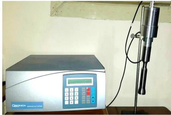
**Fig. 2.** The ultrasonicator probe
