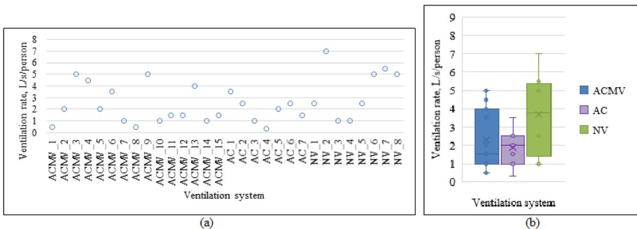
**Fig. 2.** Ventilation rate. (a) Ventilation rate at 30 CCCs and (b) Categorized by ventilation system
