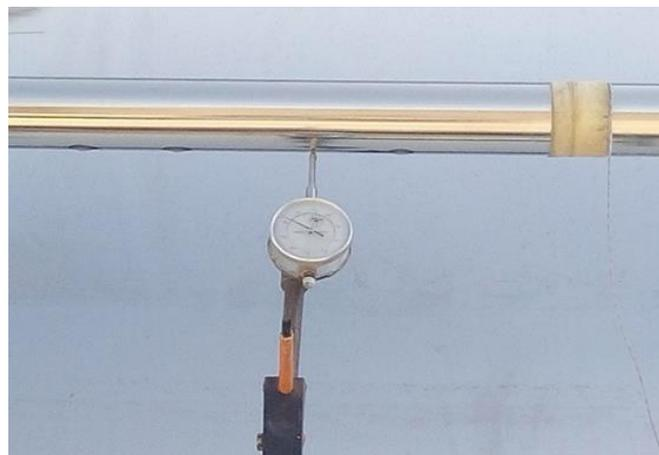
Fig. 9. Dial gauge on the mid length of the receiver tube
