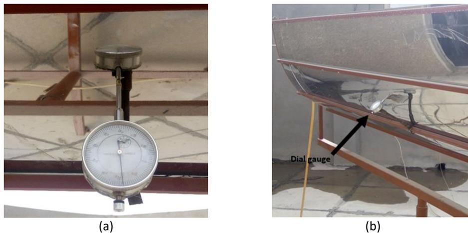
**Fig. 7.** (a) dial gauge, (b) PTC with dial gauge
