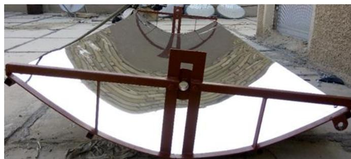
**Fig. 5.** Parabolic trough structure with plate
