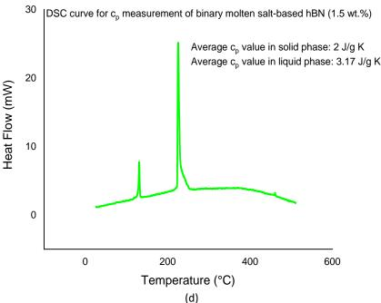
**Fig. 2.** DSC curve for  $c_p$  measurements of (a) binary molten salt (b) binary molten salt-based hBN nanocomposite (0.5 wt.%) (c) binary molten salt-based hBN nanocomposite (1 wt.%) (d) binary molten salt-based hBN nanocomposite (1.5 wt.%)
