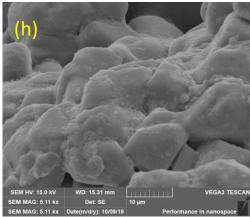
**Fig. 1.** Scanning electronic microscopy (SEM) images for (a, b) pure binary molten salt (c,d) synthesized binary molten salt-based hBN nanocomposite with loading concentration of 0.5 wt.% (e,f) synthesized binary molten salt-based hBN nanocomposite with loading concentration of 1 wt.% (g,h) synthesized binary molten salt-based hBN nanocomposite with loading concentration of 1.5 wt.%
