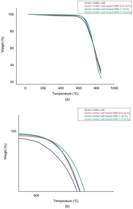
**Fig. 3.** Thermal stability measurements of binary molten salt and binary molten salt-based hBN nanocomposites in three different concentrations (a) TGA curve for all samples (b) enlarged area of beginning of decomposition in TGA curve
