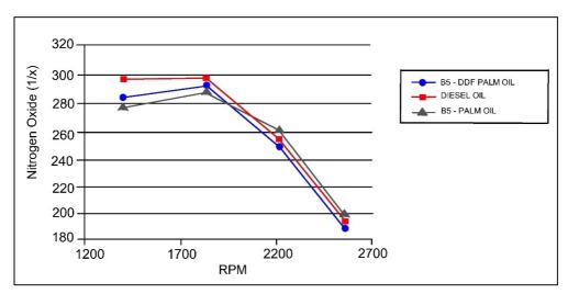
Figure 11: Nitrogen oxide against engine speed (RPM) for various fuels
