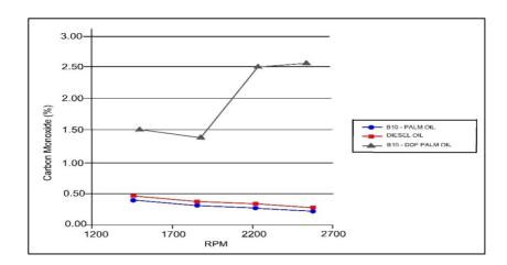
Figure 9: Carbon monoxide against engine speed (RPM) for various fuels
