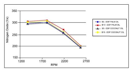
**Figure 10:** Nitrogen oxide against engine speed (RPM) for various blends of biodieselnatural gas
