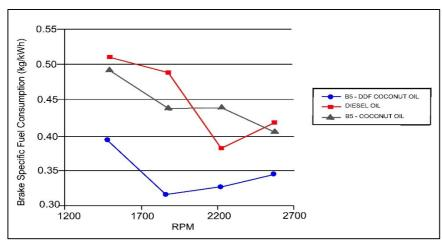
Figure 5: Brake specific fuel consumption against engine speed (RPM) for various fuels
