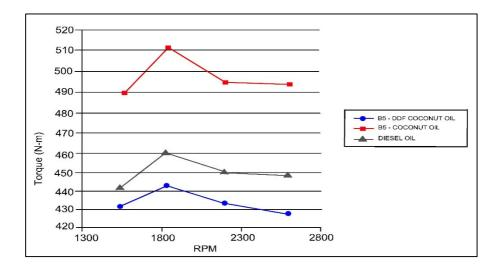
Figure 3: Torque against Engine Speed (RPM) for various fuels
