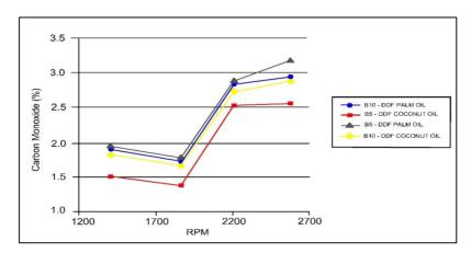
**Figure 8:**Carbon monoxide against engine speed (RPM) for various blends of biodieselnatural gas
