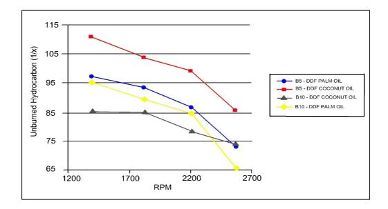
Figure 12: Unburned hydrocarbon emission against engine speed (RPM) for various blends of biodiesel-natural gas
