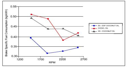
Figure 5: Brake specific fuel consumption against engine speed (RPM) for various fuels
