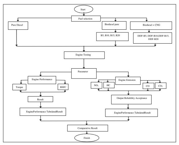
Figure 1: Flow chart of the entire step of experiment
