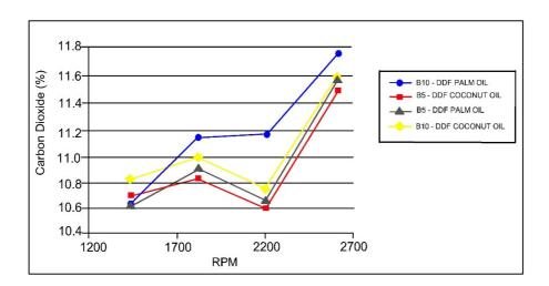
Figure 6: Carbon dioxide against engine speed (RPM) for various blend biodiesel-natural gas.
