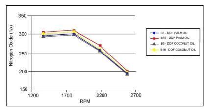
Figure 10: Nitrogen oxide against engine speed (RPM) for various blends of biodieselnatural gas
