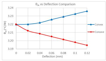
Fig. 8.  $\Theta_{JA}$  vs Deflection Simulation Data Comparison
