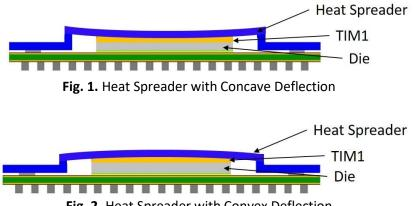
Fig. 2. Heat Spreader with Convex Deflection
