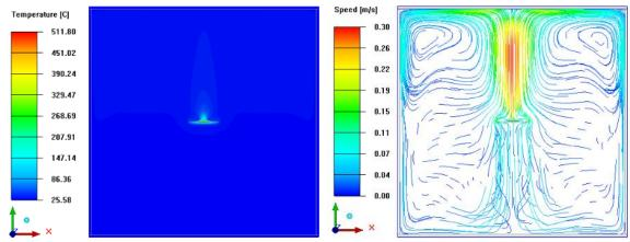
Fig. 7.  $\Theta_{JA}$  Simulation Temperature Distribution (right) and Airflow Pattern (left)
