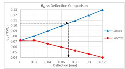
Fig. 12.  $\Theta_{JC}$  vs Deflection Simulation Data Comparison
