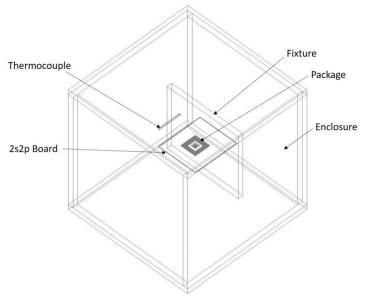
Fig. 4.  $\Theta_{JA}$  Simulation Modelling
