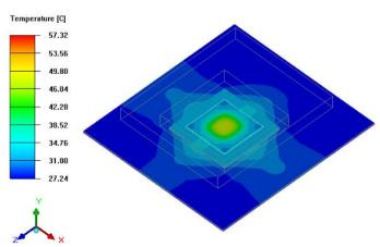
**Fig. 11.**  $\Theta_{JC}$  Simulation Board with Package Temperature Distribution
