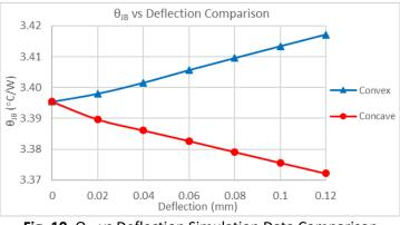
Fig. 10.  $\Theta_{JB}$  vs Deflection Simulation Data Comparison
