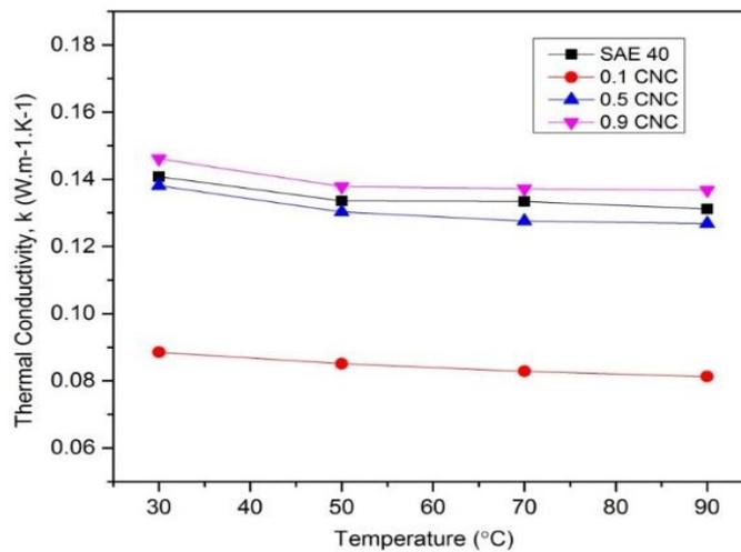
Fig. 5. Thermal conductivity of CNC at different concentration
