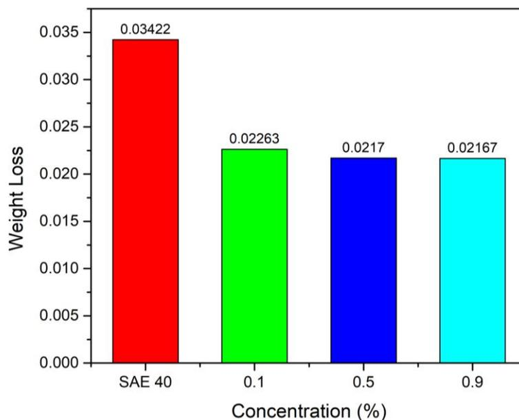
**Fig. 3.** Wear loss after tribology testing
