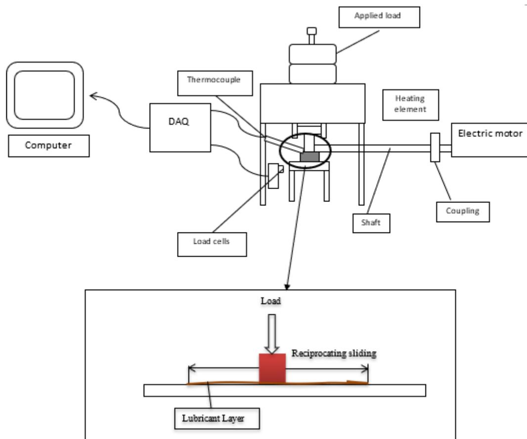
**Fig. 1.** Tribology testing setup
