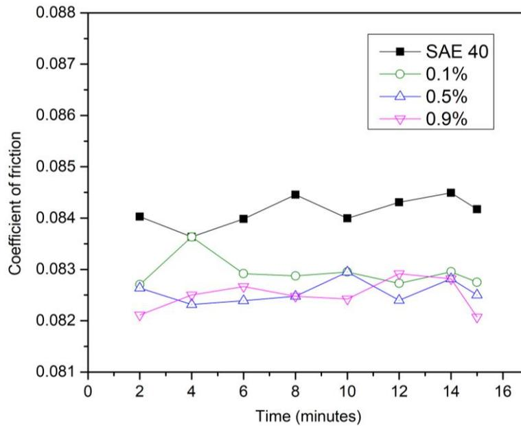
**Fig. 2.** Coefficient of friction versus time for CNC-CuO
