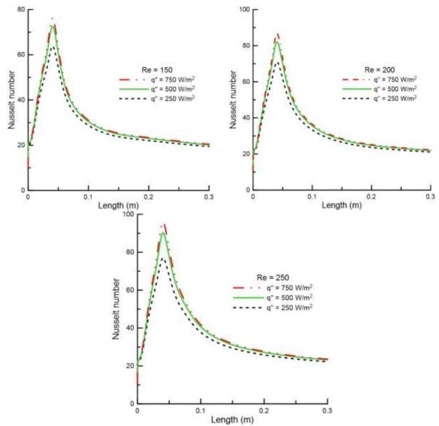
**Fig. 10.** The relation between heat transfer and streamwise direction (x) with different Reynolds number and heat fluxes for case 1
