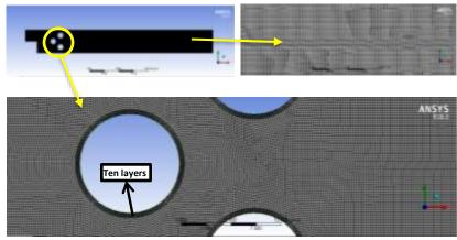
Fig. 3. Grid structure for backward step with three cylinders
