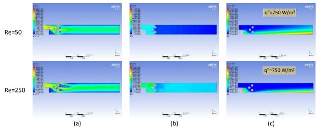
Fig. 5. Counters of (a) velocity (b) pressure and (c) temperature at selected Reynolds number and heat flux for case 1
