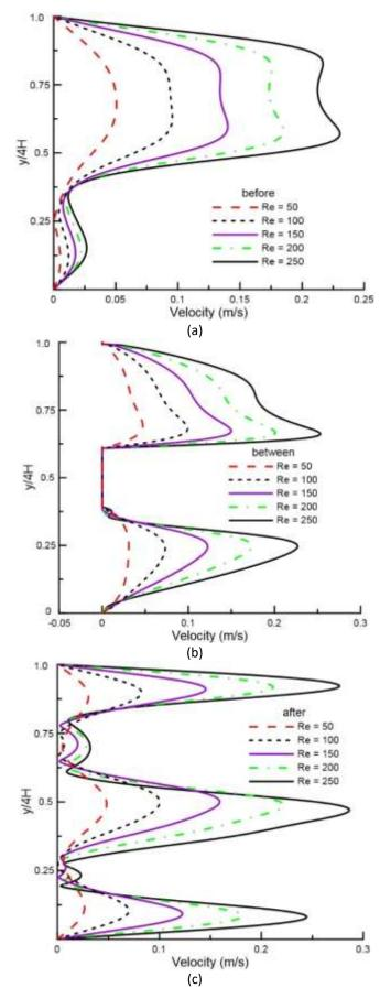
**Fig. 8.** Velocity profile at three streamwise locations, (a) x = 0.01 m, (b) x = 0.03 m, and (c) x = 0.05 m
