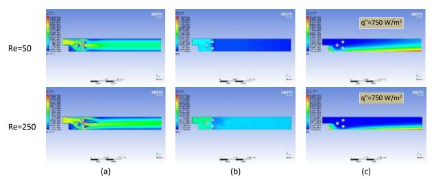
Fig. 6. Counters of (a) velocity (b) pressure and (c) temperature at selected Reynolds number and heat flux for case 2
