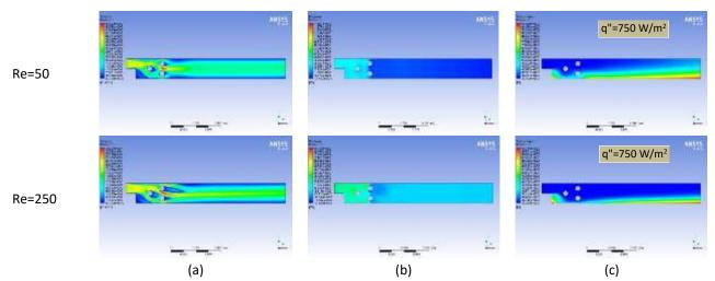
**Fig. 7.** Counters of (a) velocity (b) pressure and (c) temperature at selected Reynolds number and heat flux for case 3
