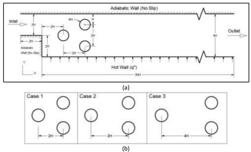
**Fig. 1.** Schematic diagram of backward facing step (a) the physical domain, (b) three cases for the location of the cylinders
