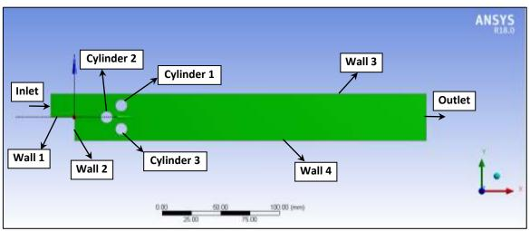
Fig. 2. Schematic description of physical domain with boundary conditions
