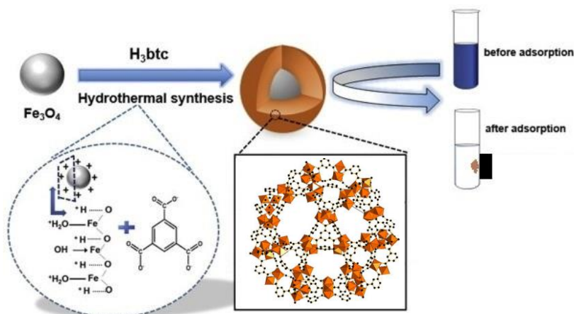
Fig. 4. Schematic diagram of dye removal by Fe 3 O 4 @MIL-100(Fe) core-shell
