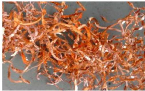
**Figure 1:** Copper Mesh used as regenerator material.
