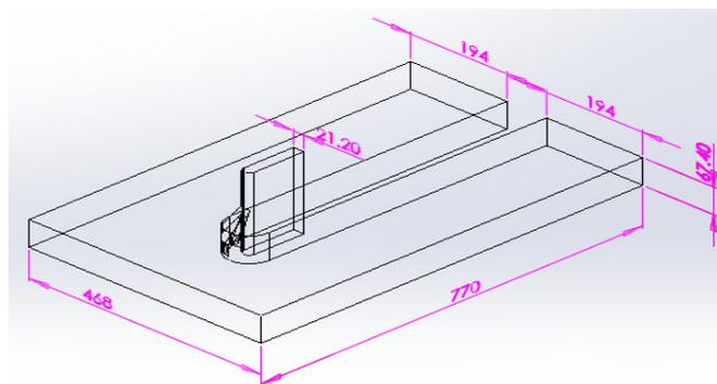
**Figure 1:** Schematic for the leading edge
