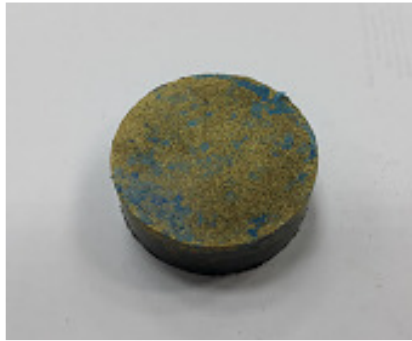
Figure 3: Briquette contains mixture of pulverized EFB and polyethylene plastics (weight ratio 85:15), produced under temperature of 190°C.
