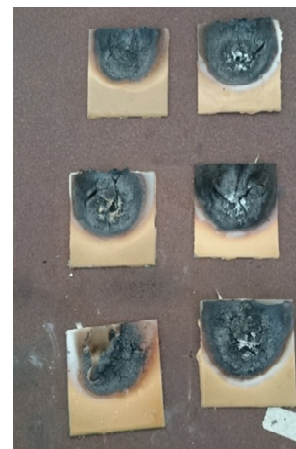
Figure 8: Intumescent coated steel, 10 cm X 10 cm samples after fire resistance test
