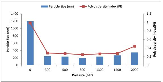
Figure 1: Effect of HPH pressure on ZO-NLC properties
