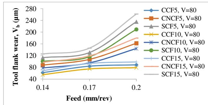
**Figure 11:** Variation of tool flank wear with feed
