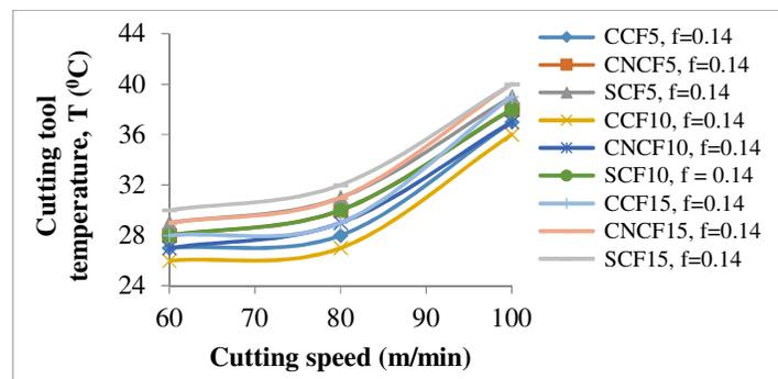
**Figure 8:** Variation of cutting tool temperature with cutting speed
