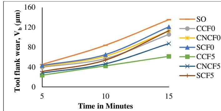
**Figure 4:** Variations of tool flank wear with time
