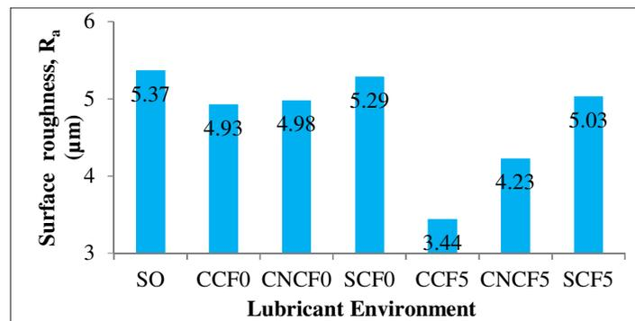
**Figure 5:** Variation of surface roughness ( $R_a$ ) at different lubricating conditions
