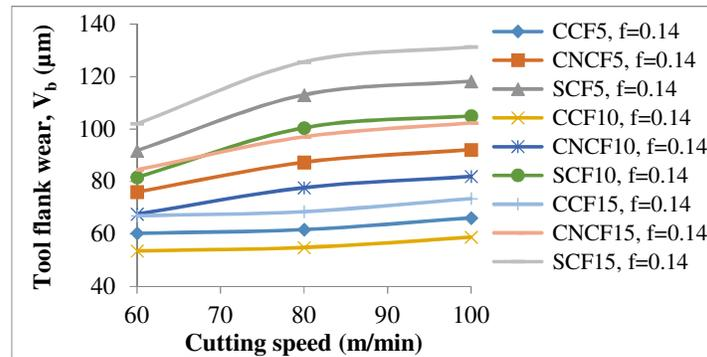
**Figure 10:** Variation of tool flank wear with cutting speed
