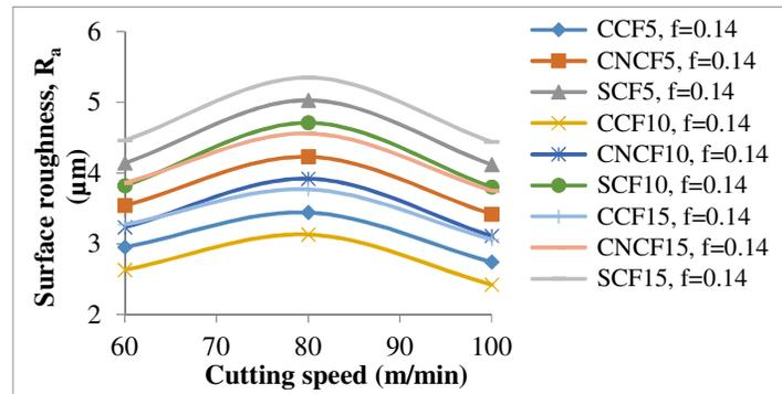
**Figure 12:** Variation of surface roughness ( $R_a$ ) with cutting speed
