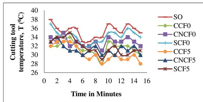
**Figure 3:** Variation of cutting tool temperature with machining time
