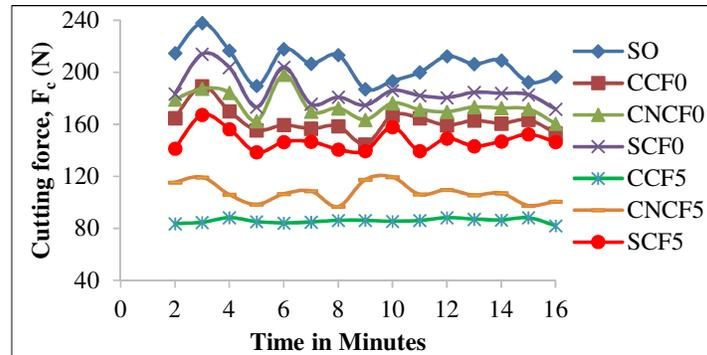
**Figure 2:** Variation of cutting force with machining time
