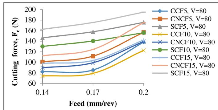
**Figure 7:** Variation of cutting force with feed
