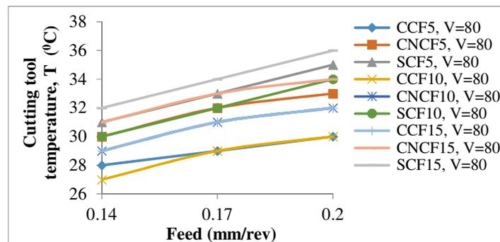
**Figure 9:** Variation of cutting tool temperature with feed
