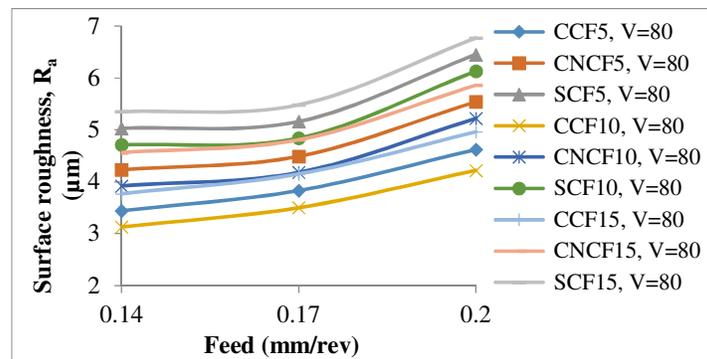
**Figure13:** Variation of surface roughness ( $R_a$ ) with feed
