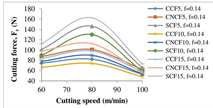
**Figure 6:** Variation of cutting force with cutting speed
