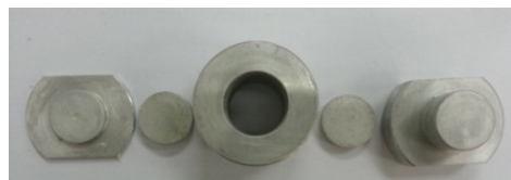
Figure 1. Aluminium mould used to produces sample.
