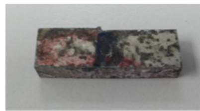
Fig. 3. Reference sample after SST
