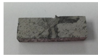
Fig. 5. Cold sprayed sample after SST
