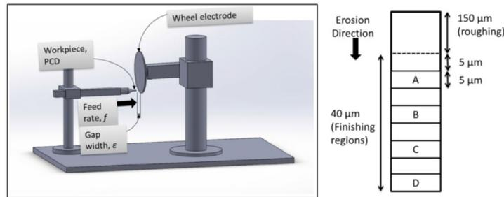
**Fig. 1.** Experimental setup and procedure
