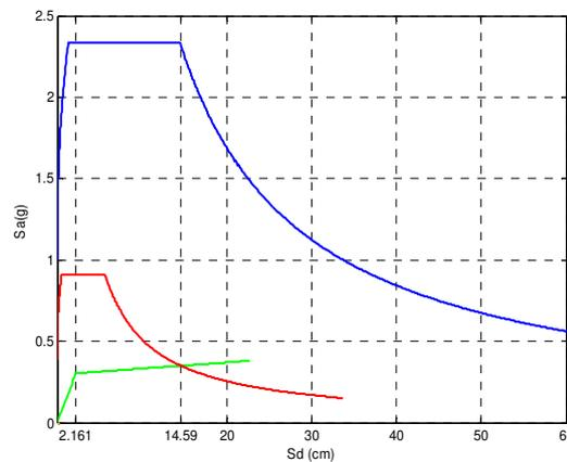
**Fig. 9.** Performance Point Determination
