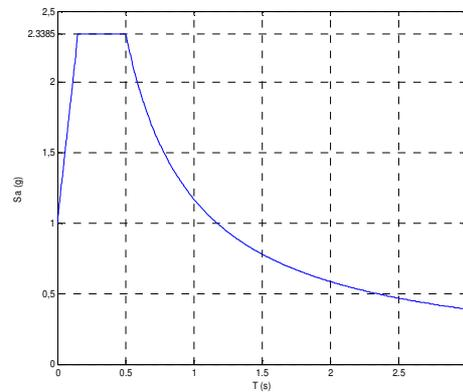
**Fig. 2.** Elastic Spectrum of RPA99 for Mobile Site
