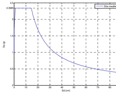
**Fig. 5.** Spectrum elastic format Acceleration-Displacement for a movable site
