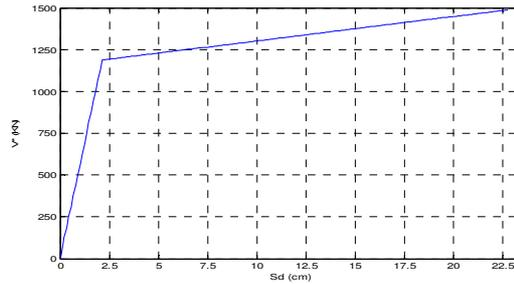
**Fig. 6.** The Push Over curve for a system
