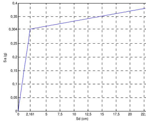
**Fig. 7.** Capacity curve
