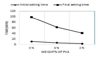
**Fig. 5.** Influence of PVA concentration on the setting times of CPC paste [49]
