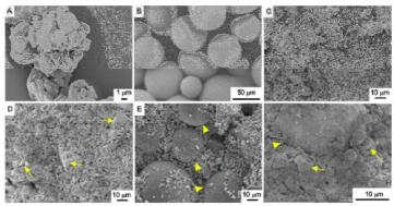
**Fig. 3.** Microscopic SEM micrograph of (A) BG granulate, (B) dense PLGA-microparticles, (C) CPC, (D) CPC/BG30, (E) CPC/PLGA and (F) CPC/PLGA/BG30. BG (arrow) and PLGA-microparticles (arrowheads) are indicated in the SEM micrograph [39]
