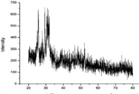
**Fig. 4.** X-ray diffraction pattern of injectable strontium-containing calcium phosphate cement with collagen [41]
