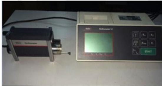
Fig. 2. Perthometer M1 device with stylus
