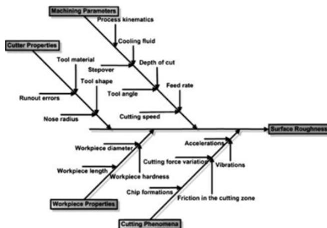
Fig. 2. Surface roughness Fishbone diagram parameters [8]
