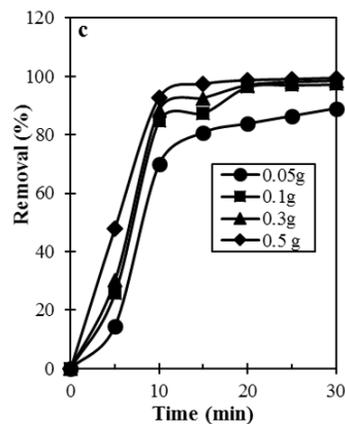
Fig. 7. Effect of adsorbent dosage on removal efficiency of 2-CP
