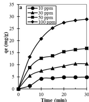
Fig. 5. Effect of contact time on adsorption at different concentrations
