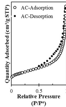
Fig. 2. N<sub>2</sub> adsorption-desorption isotherm for AC
