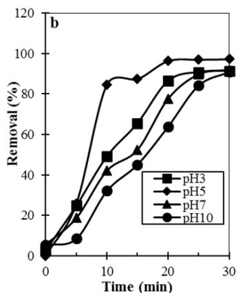
Fig.6. Effect of pH on removal efficiency of 2-CP
