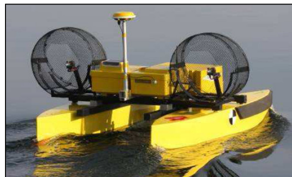
Figure 5: The robot-boat CatOne using the concept of catamaran for shallow water hydrography.
