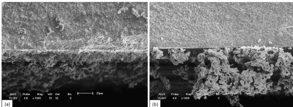
**Figure 1:** SEM images of the cathode-electrolyte interfaces of LSCF-SDC-Ag/SDC (a) and LSCF-SDC/SDC (b) [5]
