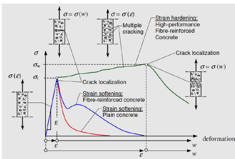
Fig. 4. Cementitious composites tensile reaction categorisation [32]
