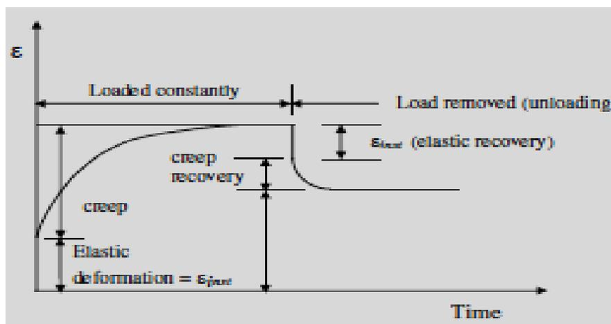
Fig.3. Strain-time relationship of concrete under sustained loading
