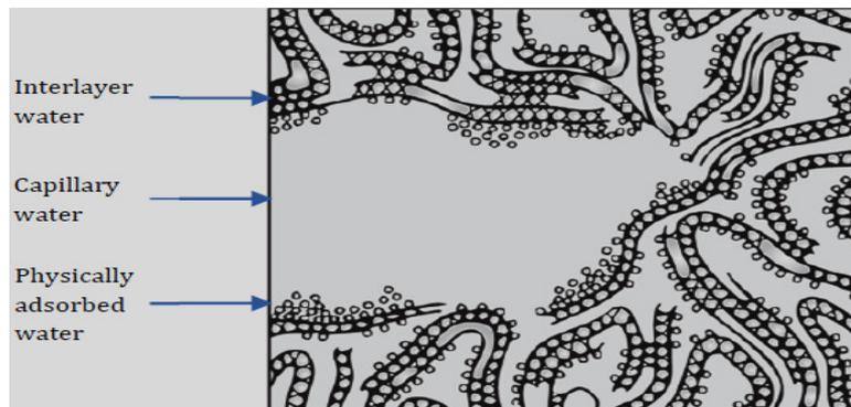
Fig. 1. Hydrated cement paste and water type in it [10]
