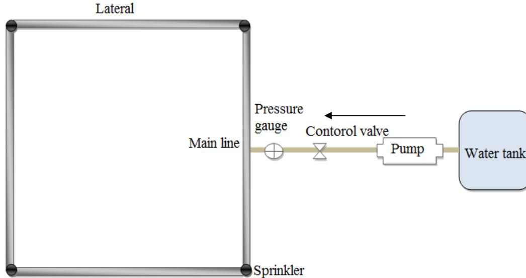
**Figure 3:** Schematic diagram of the sprinkler irrigation system
