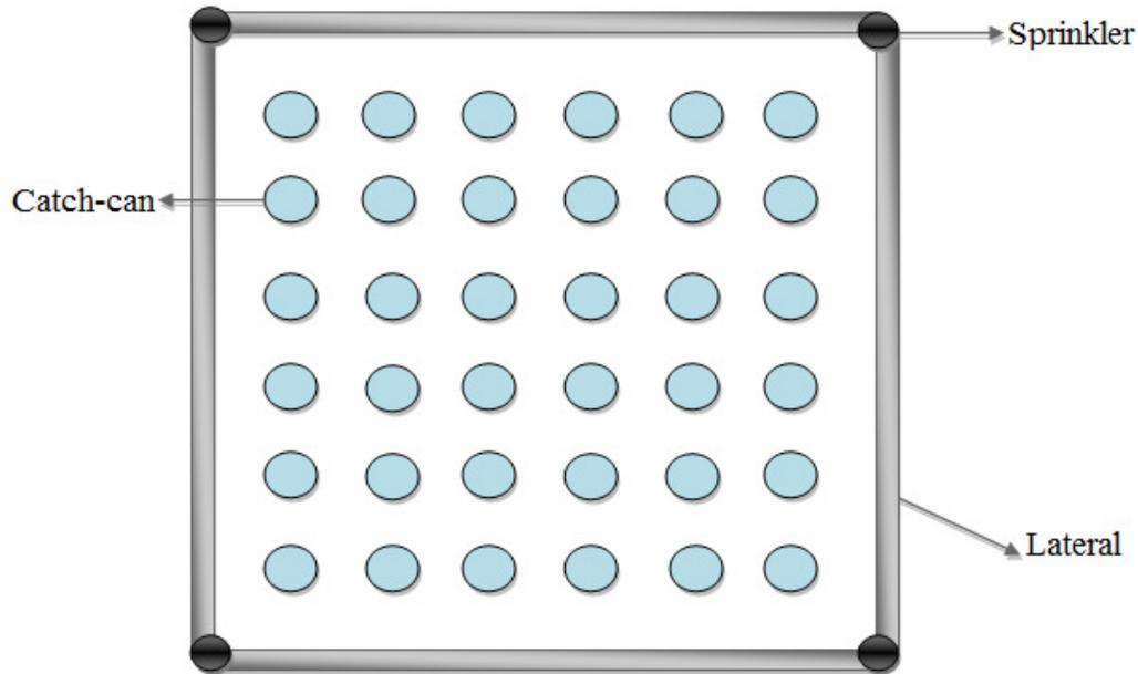
**Figure 4:** Catch-cans arrangement for the block irrigation test
