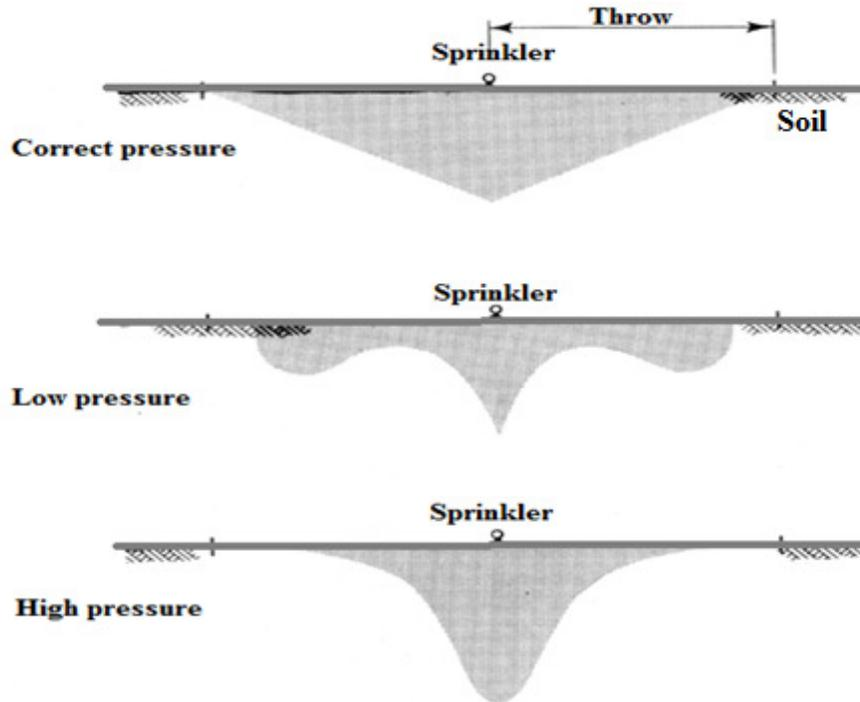
**Figure 1:** The effect of pressure on water distribution uniformity
