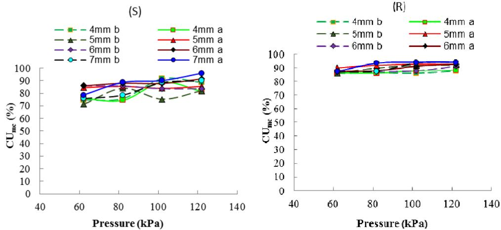
**Figure 8:** Christiansen's coefficient of uniformity of soil moisture content ( $CU_{mc}$ ) at 0-5 cm depth before (b) and 10 min after (a) irrigation event for different nozzle diameters (mm) and pressures (KPa) at 1.0 m riser for (S) a square system of 12x12 m and (R) a rectangular system of 10x12 m.
