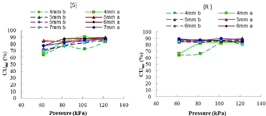
**Figure 7:** Christiansen's coefficient of uniformity of soil moisture content ( $CU_{mc}$ ) at 0-5 cm depth before (b) and 10 min after (a) irrigation for different nozzle diameters (mm) and pressures (kPa) at 0.75 m riser for (S) a square system of 12x12 m (R) and a rectangular system of 10x12 m.
