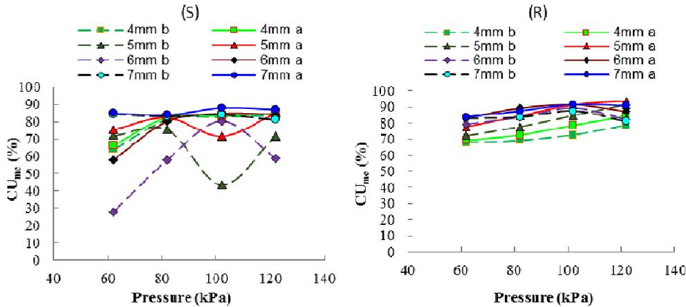
**Figure 6:** Christiansen's coefficient of uniformity of soil moisture content ( $CU_{mc}$ ) at 0-5 cm depth before (b) and 10 min after (a) irrigation for different nozzle diameters (mm) and pressures (kPa) at 0.5 m riser for (S) a square system of 12x12 m and (R) a rectangular system of 10x12 m
