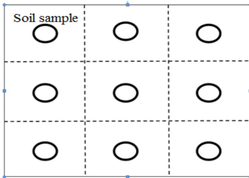
**Figure 5:** Sampling locations of grid samples for soil moisture content measurements at the field site
