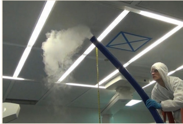
Figure 3: Airflow visualization smoke study [10]
