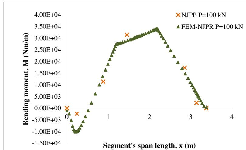
**Figure 8:** Bending moment for pin-roller support condition (NJPR) with numerical modelling result (FEM-NJPR) of single segment
