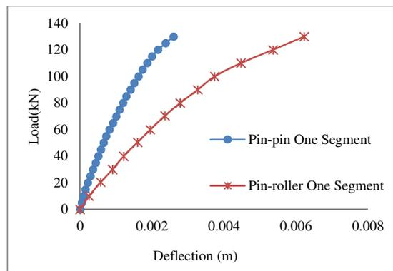
Figure 5: Load vs. deflection at mid span of segment
