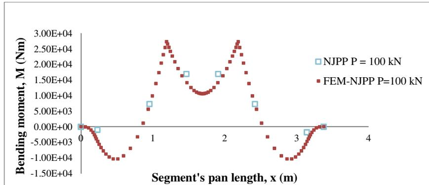
**Figure 7:** Bending moment for pin-pin support condition (NJPP) with numerical modelling result (FEM-NJPP) of single segment
