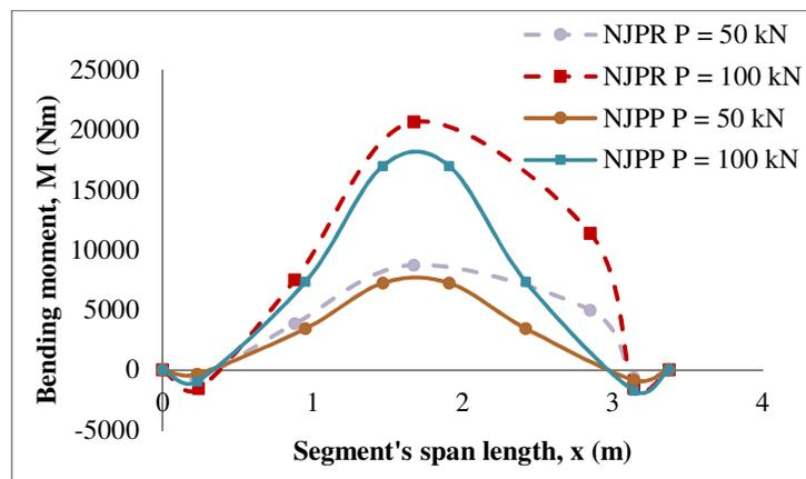
Figure 6: Bending moment for non-jointed pin-roller test (NJPR) and non-jointed pin-pin test (NJPP) of single segment
