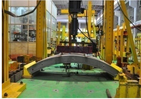
**Figure 3:** Test arrangement of pin-pin support for single segment
