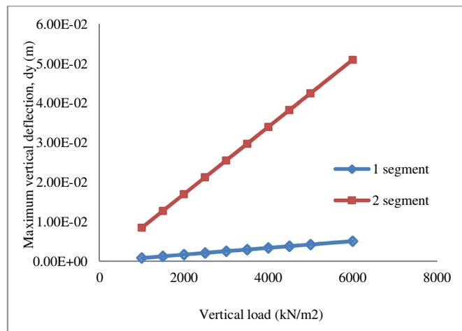
**Figure 2:** Load - deflection curves of one segment and dual jointed segment
