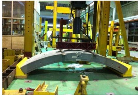
**Figure 4:** Test arrangement of pin-roller support for single segment
