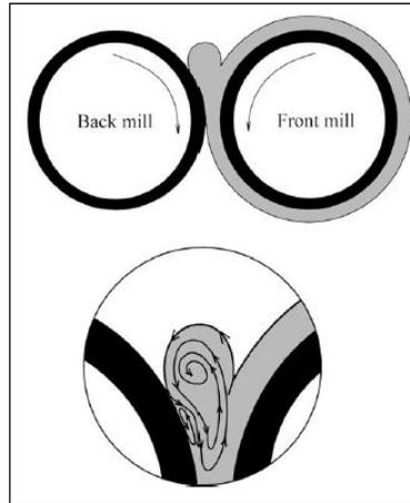
**Figure 2:** Conceptual view of two-roll mills [4]
