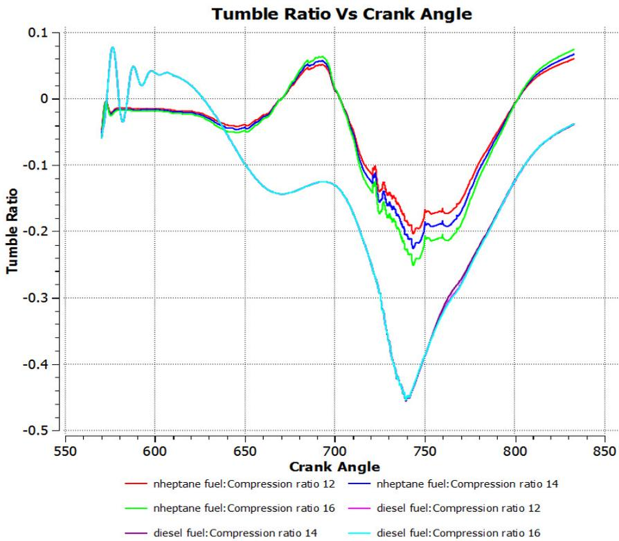
Fig. 7. Diesel, n-Heptane: Tumble ratio vs crank angle
