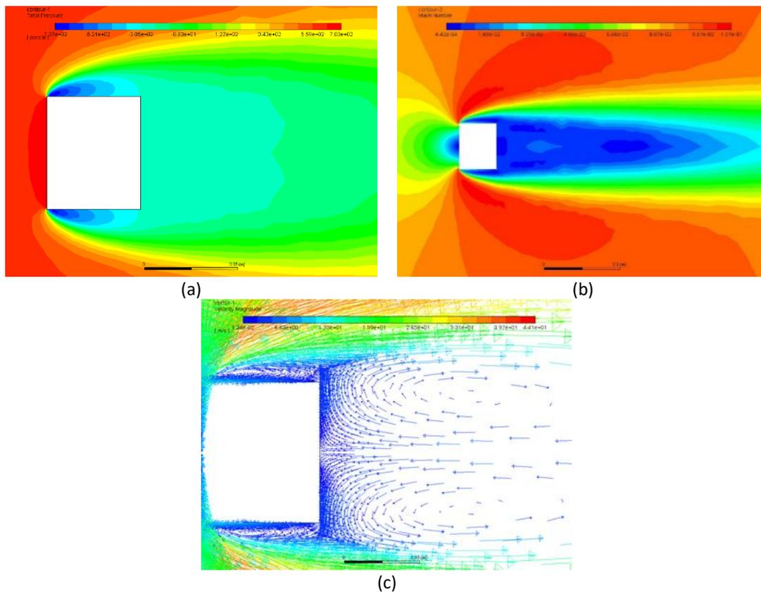
**Fig. 7.** Velocity = 24.8 m/s (a) total pressure contour (b) velocity contour (c) vector
