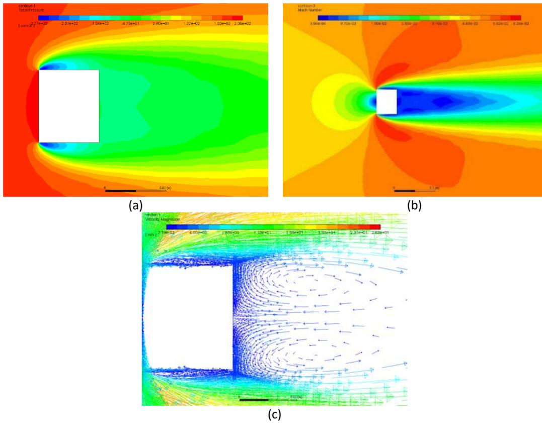
**Fig. 6.** Velocity = 16.18 m/s (a) total pressure contour (b) velocity contour (c) vector
