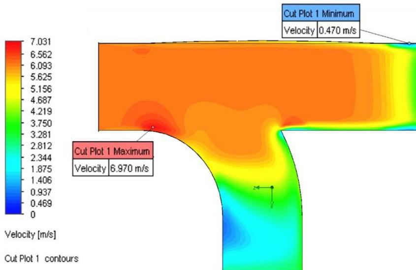
**Fig. 8.** Air velocity variance in wye-tee duct with protrusion design
