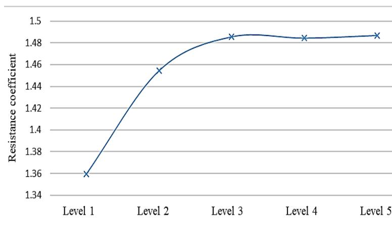
**Fig. 4.** Mesh density vs Resistance coefficient,  $C_b$
