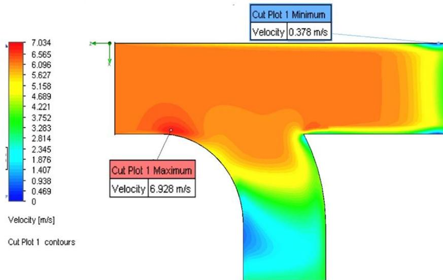
Fig. 10. Air velocity variance in traditional wye-tee duct
