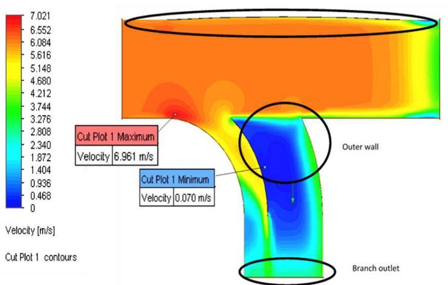
Fig. 11. Air velocity variance in wye-tee duct with protrusion and guide vane at optimum location
