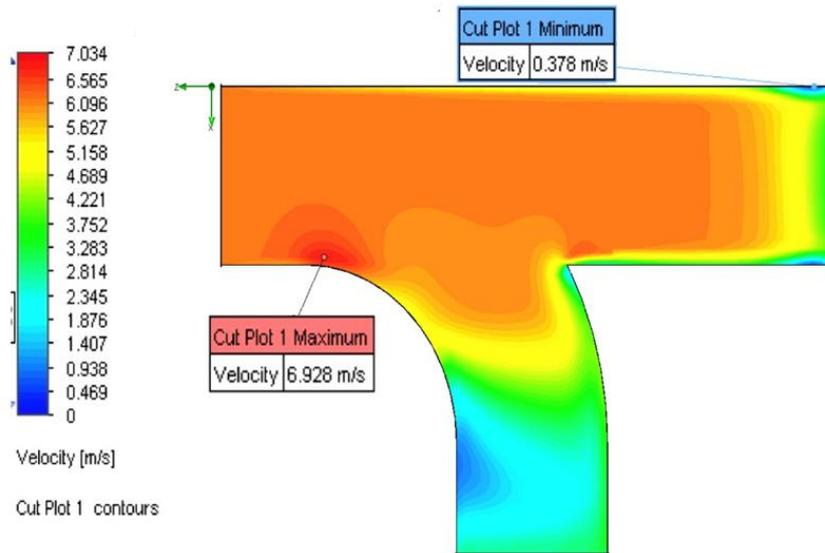
**Fig. 7.** Air velocity variance in standard wye-tee duct
