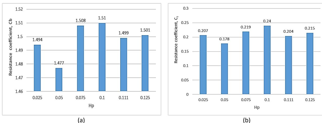
**Fig. 6.** Height of protrusion,  $H_p$  vs Resistance coefficient, (a)  $C_b$  and (b)  $C_s$
