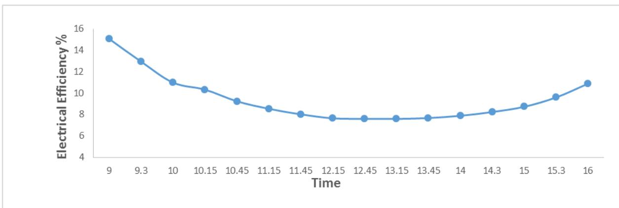
**Fig. 6.** Simulation validation on the hourly variation of electrical efficiency of hybrid PVT air collector
