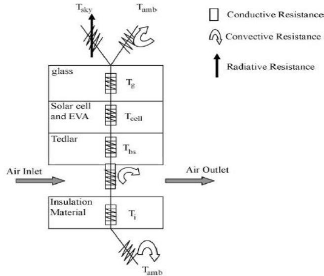
**Fig. 1 (a)** Cross sectional view of the PVT air collector[18]
