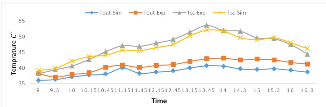
**Fig. 3.** Comparison of experimental and simulation of solar cell temperature and outlet air temperature of hybrid PVT air collector
