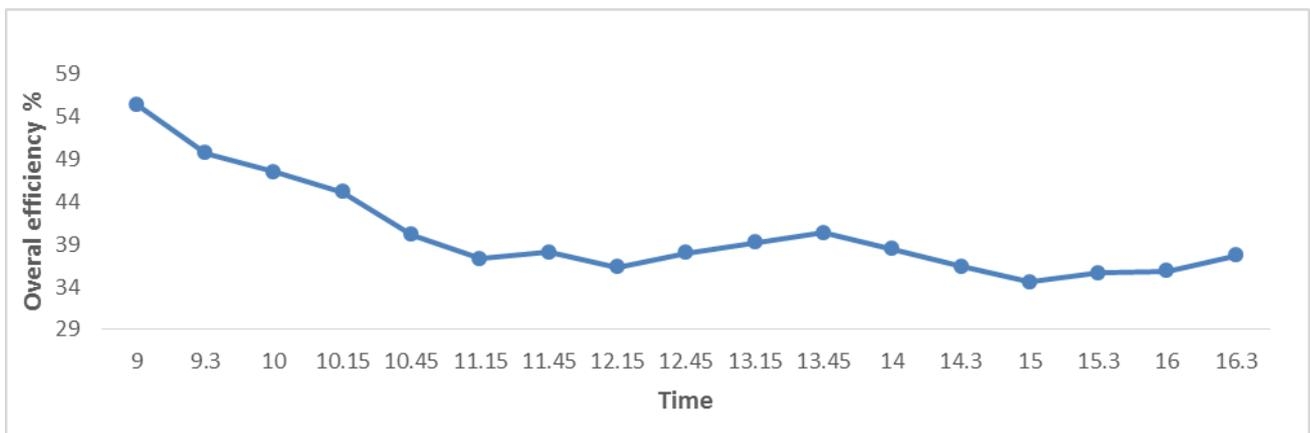
**Fig. 7.** Simulation validation on the hourly variation of overall efficiency of hybrid PVT air collector
