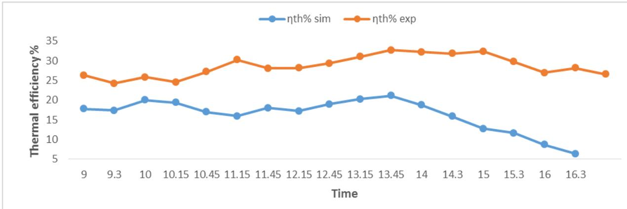
Fig. 4. Comparison of experimental and simulation thermal efficiency of hybrid PVT air collector
