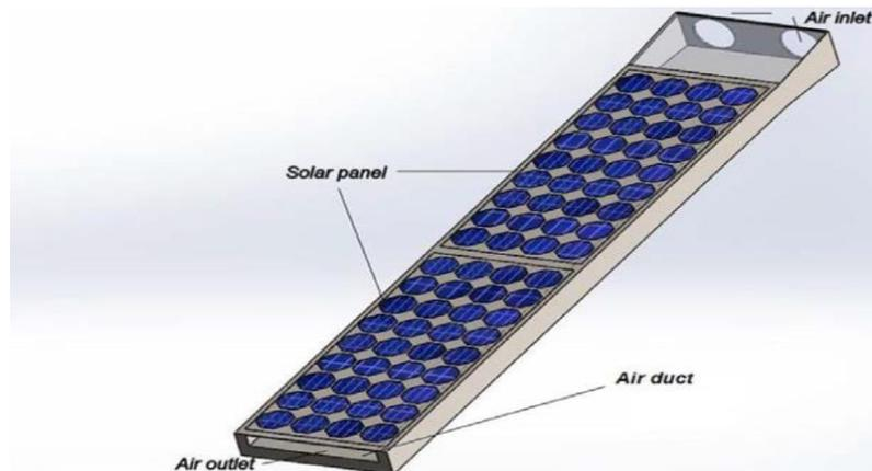
**Fig. 2.** Geometric model of hybrid PVT air collector
