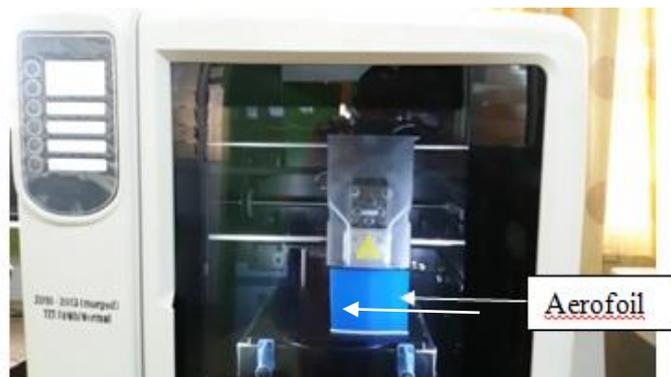
**Fig. 4.** The U-Print SE Plus printer producing the airfoil model
